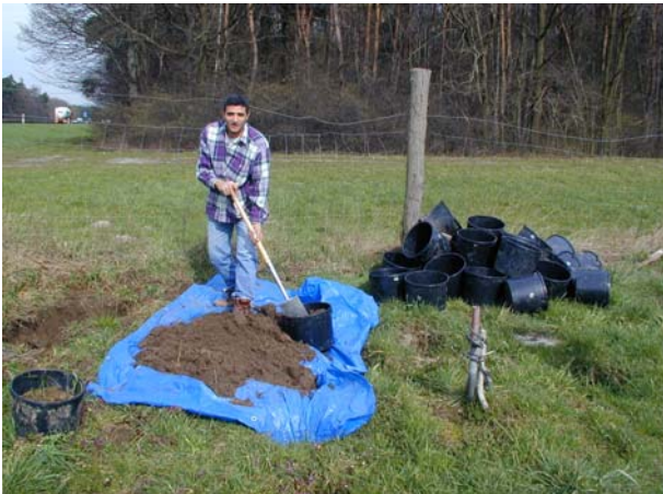
Picture (1): Homogenization and filling of the soil in pots at the highway site for field experiments.
