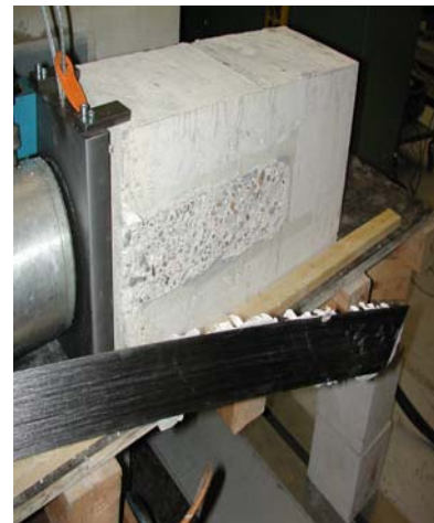
Figure 4.11: Failure shape: AAC-blocks strengthened with GFRP-sheet (a); Concrete-blocks strengthened with CFRP-sheet failure shape (b).
