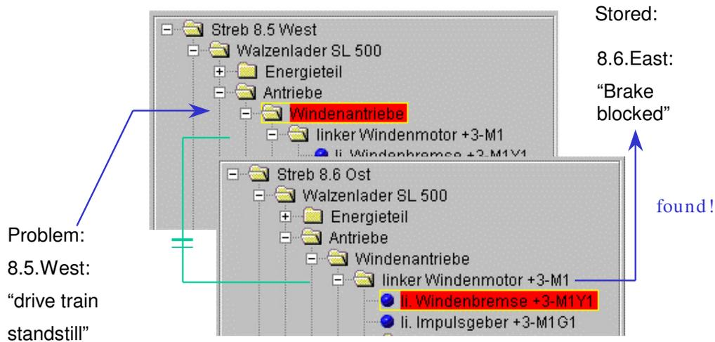
**Figure 32: Example for Ontology-Based Retrieval**
