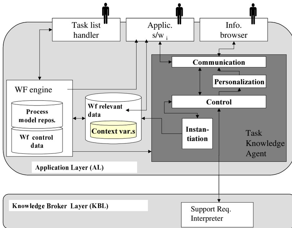
**Figure 25: Generic Architecture for Application Layer**
