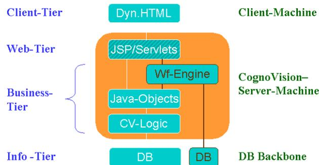
**Figure 68: Architecture of DECOR Workflow Engine**
