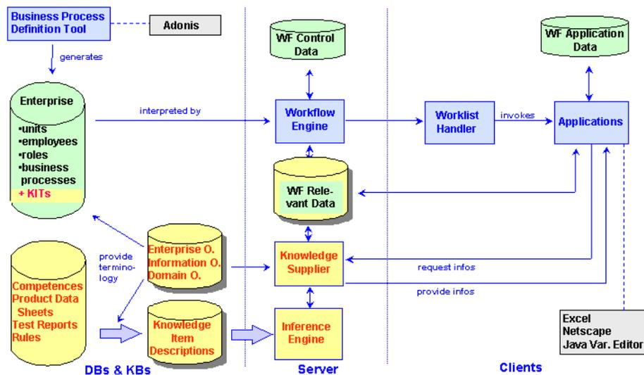
**Figure 18: The KnowMore System has a Web-Enabled C/S- Architecture**
