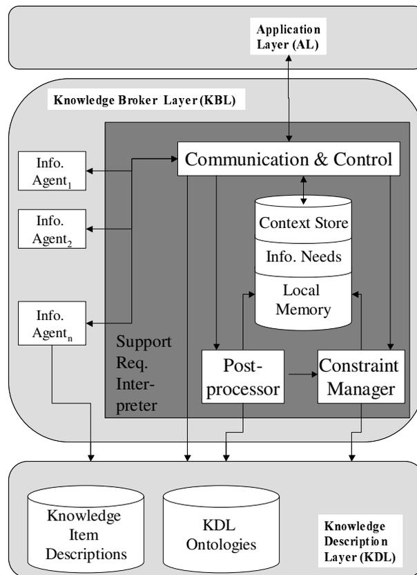
**Figure 30: Generic Architecture for Support Request Interpreter**
