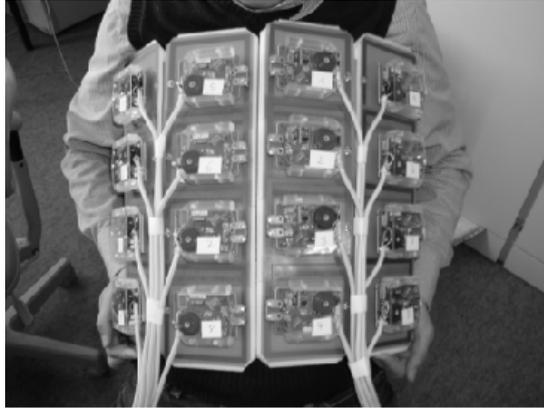
**Fig. 3.12** Experimental 32 element coil array
