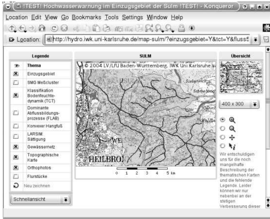
Figure 4.37.: Test implementation of an application based on the UMN map server to provide information about the soil moisture state of a small catchment.
