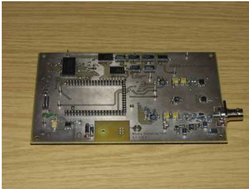
Figure 3.1.: OBSERVER V2, second prototype for a new Time-Domain-Reflectometer based on Delta Modulation and Direct Digital Synthesis.
