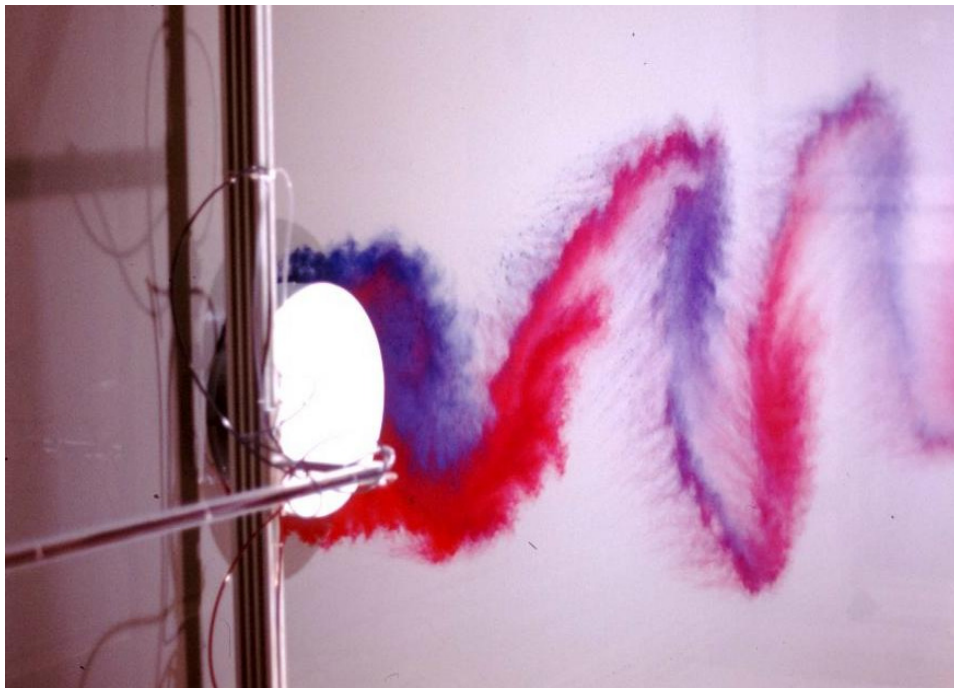
(b) Vortex street-like instability in shallow turbulent wake
