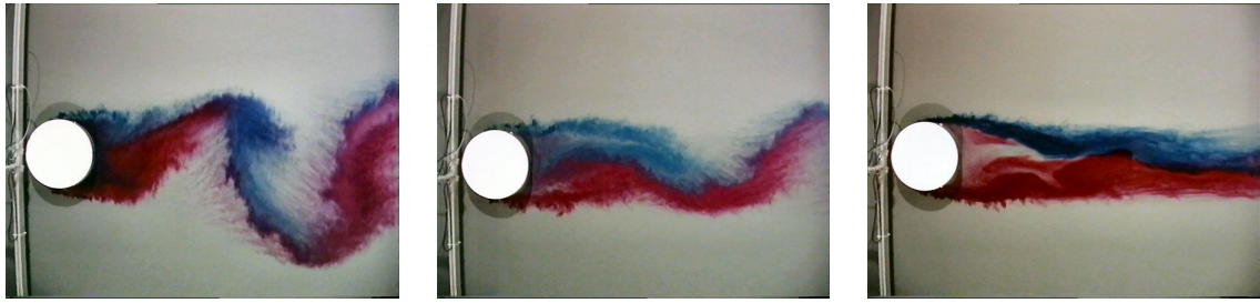
(a) VS - vortex street-like wake (b) UB - unsteady bubble wake (c) SB - steady bubble wake
