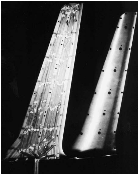
Fig. 2.33 : Static pressure bore holes in a wing model
