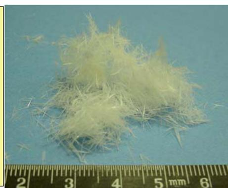
Figure 10: Needle shaped crystals from UP degradation gas.
