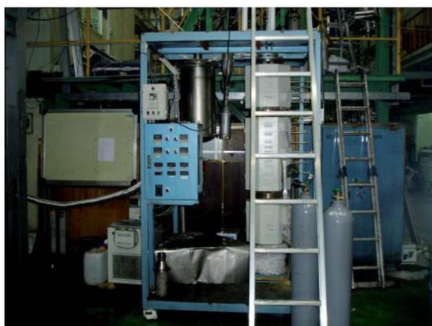
Figure 1: Bubbling fluidized bed reactor of this experiment.
