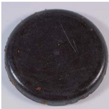
Figure 3: Recycled plastic made of depolymerized material of waste FRP.
