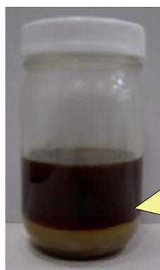
Figure 9: Precipitate in the UP degradation oil.
