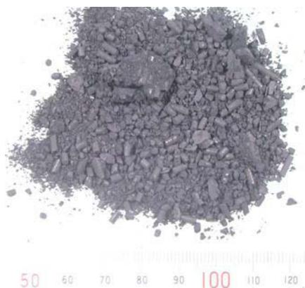
Figure 7: Photograph of catalyst after 40 days operation.
