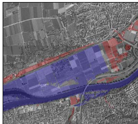
Figure 5.6. Inundation area overlaid over aerial photograph in a section of the Heilbronn sub-reach (blue = Inundation, red = potential inundation)
