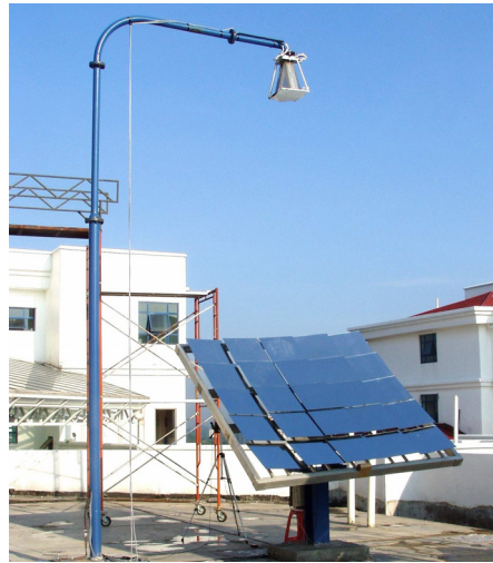
FIGURE 6: The prototype of 300 concentration using CPV
