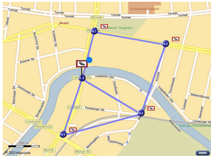
Fig. 7.5. Global view of VANET cars. Network connectivity and an emergency message with corresponding propagation symbols are displayed.
