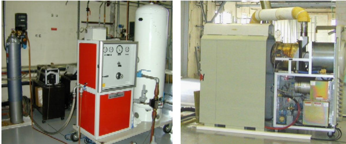
Figure 2: Microturbine test bench for performance assessment
