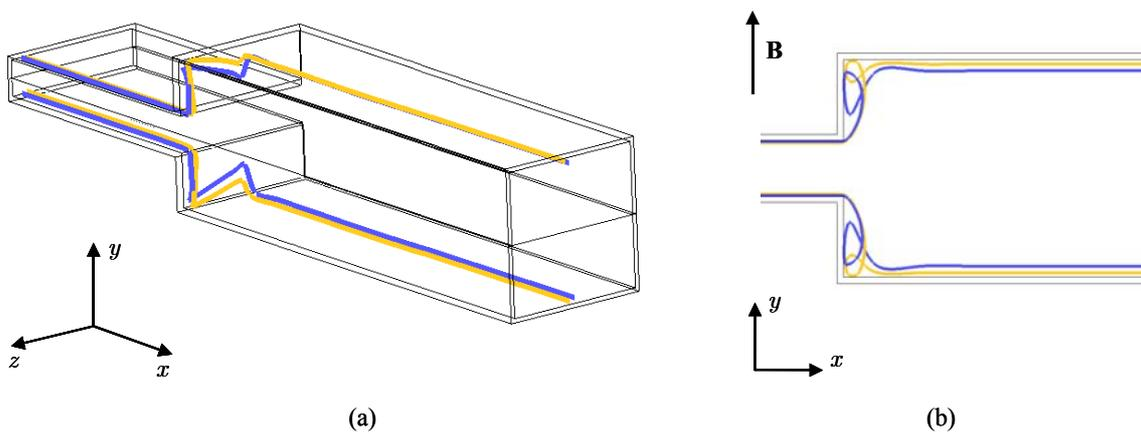
Figure 78: Flow paths for  $Ha = 400$  and  $N = 50$  that transport the fluid from the upstream side layer, close to the horizontal walls, towards the Hartmann walls and to the center of the duct forming, near the middle plane, a V-shaped trajectory.
