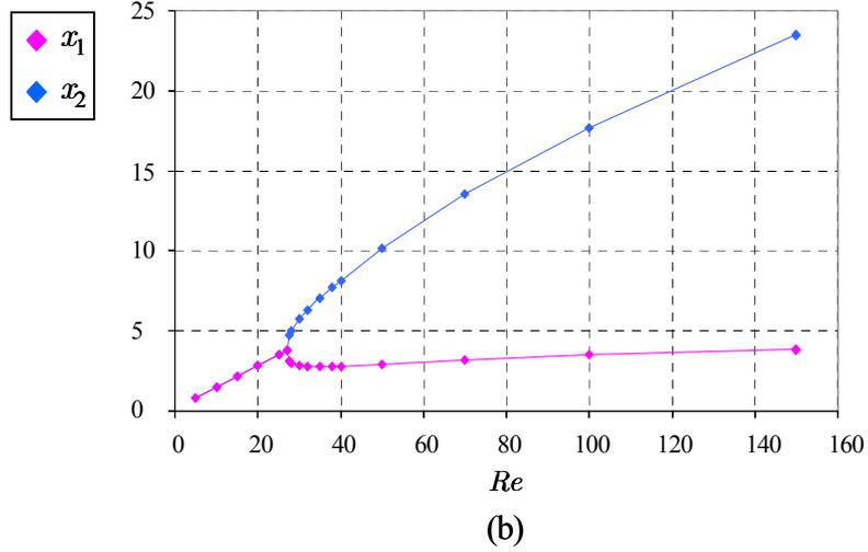
Figure 22: Locations of reattachment and separation points of recirculations on the side wall (a) and on the symmetry plane  $z = 0$  (b) as a function of Reynolds number. The black dashed line (a) indicates the axial position of the node  $N_{3s}$ .
