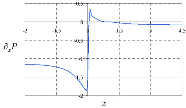
Figure 43: Axial component of pressure gradient along the axis of the duct for  $Ha = 700$ ,  $N = 4900$  and  $c = 0.1$ . The variable  $P$  is given by  $p/N$  where  $p$  is the pressure in the hydrodynamic scale.
