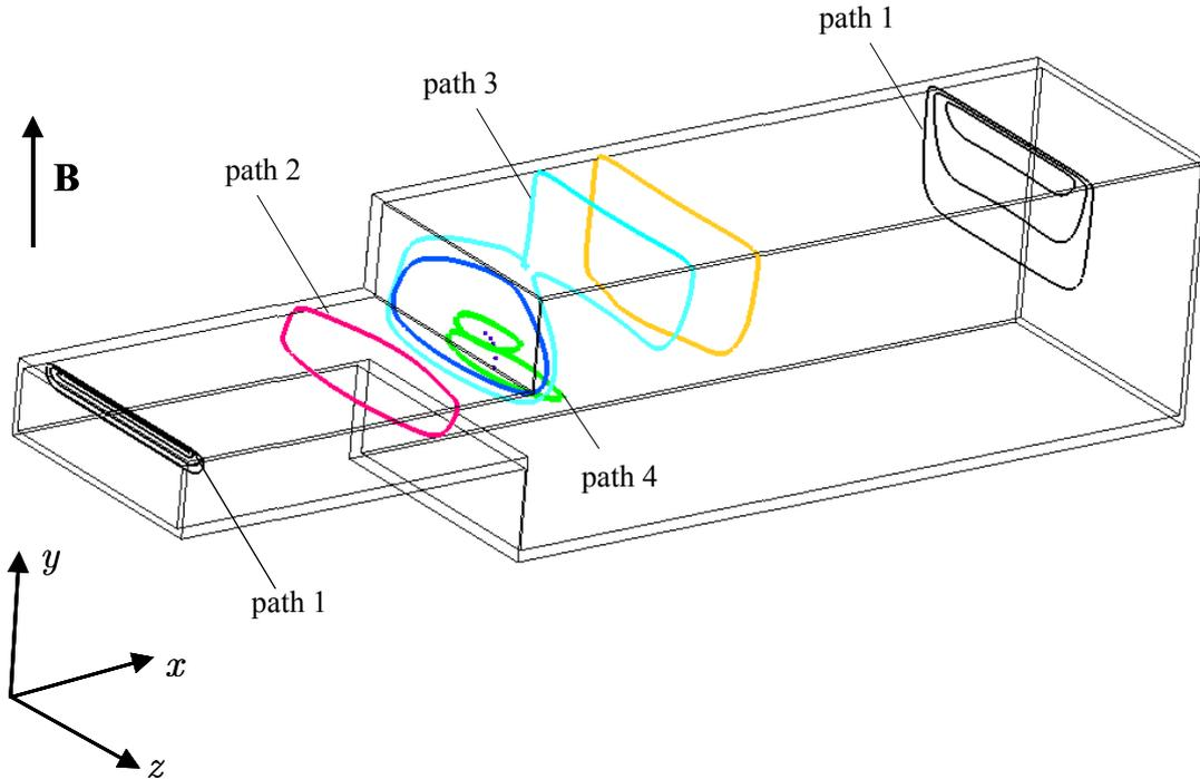
Figure 60: Current paths for the flow at  $Ha = 50$ ,  $N = 25$  and  $c = 0.1$ . The blue points indicate the line around which the core loops develop.
