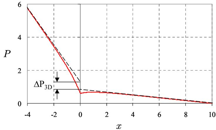
Figure 44: Pressure distribution along the axis of the duct for  $Ha = 700$  and  $N = 4900$ .  $\Delta P_{3D}$  indicates the additional pressure drop caused by the 3D current density. It is related to the pressure loss in hydrodynamic scale as  $\Delta P_{3D} = \Delta p_{3D}/N$ .
