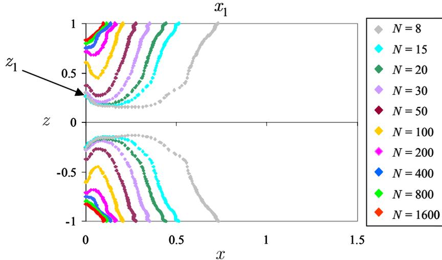
Figure 82: Lines where the  $x$ -component of the velocity is zero plotted on the Hartmann wall for  $Ha = 400$  and several interaction parameters  $N$ .  $x_1$  marks the end of the back flow region on the side wall,  $z_1$  indicates the extent of the zone of reverse flow on the expansion wall.
