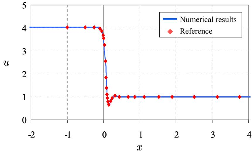
Figure 15: Velocity component  $u$  along the channel midline  $y = 0$  for  $Ha = 1000$  and  $N = 1000$ . The solution is computed on *grid D*. The symbols indicate results from the literature ( Aleksandrova et al. (2003)).
