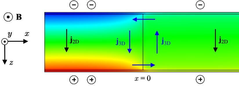
Figure 42: Schematic representation of the distribution of fully developed and induced 3D currents on the plane  $y = 0$ . The contour plots indicate the potential distribution for  $Ha = 700$  and  $N = 4900$ .
