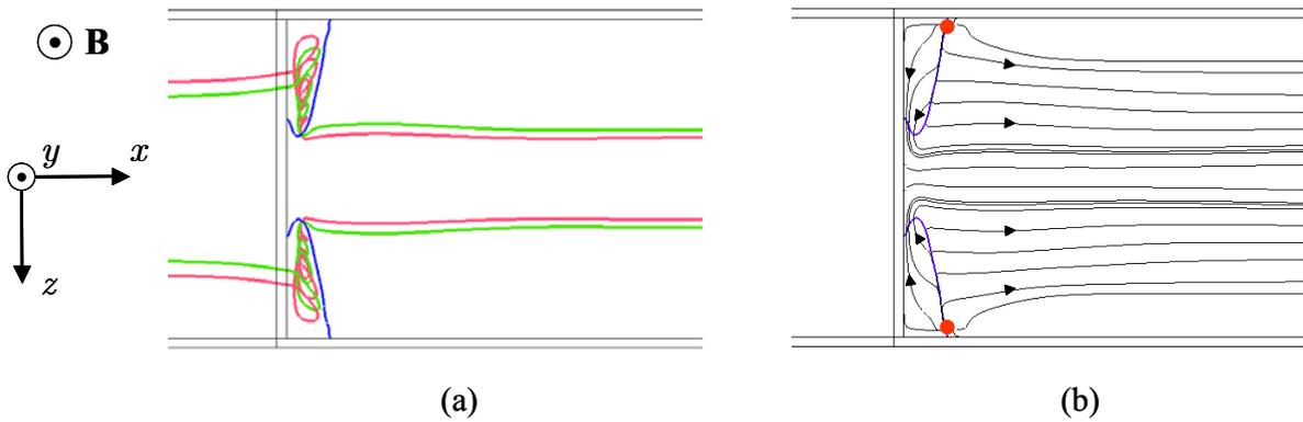
Figure 81: (a) Top view of vortices formed behind the expansion (green and red paths) for the flow at  $Ha = 400$  and  $N = 50$ . The blue curve indicates the points where the axial velocity components  $u$  becomes zero. (b) Limiting streamlines are plotted on the Hartmann wall. The red dots are critical points that act as sources of streamlines.
