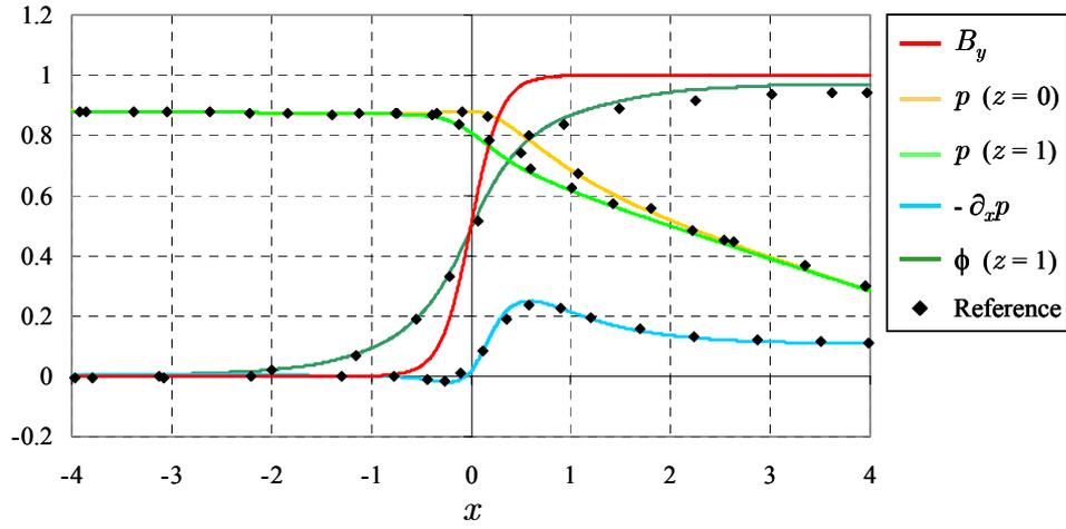
Figure 17: Characteristic quantities plotted along the axial direction for the flow in a non-uniform magnetic field at  $Ha = 50$ ,  $N = 1000$ ,  $c = 0.1$ . The symbols indicate the reference results (Sterl (1990)).
