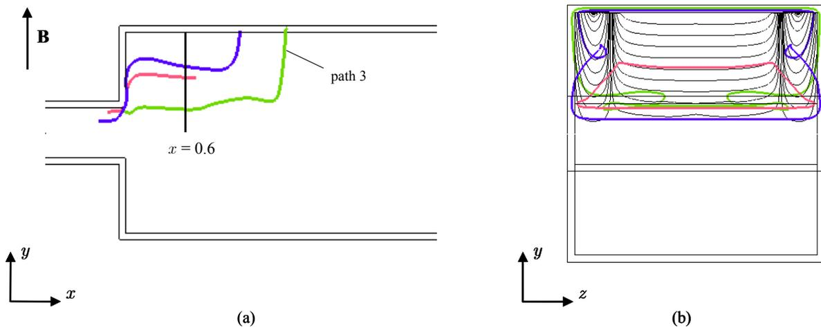
Figure 70: Current lines for  $Ha = 400$ ,  $N = 1600$  and  $c = 0.1$ . (a) The vertical line at  $x = 0.6$  indicates the plane on which pseudo streamlines are drawn. (b) Limiting streamlines are plotted in black.
