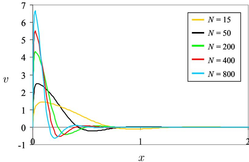
Figure 76: Vertical velocity plotted along the axial direction near the internal edge of the expansion at  $y = 0.25$ , on the middle plane at  $z = 0$  for  $Ha = 400$  and a range of the interaction parameter  $N$ .
