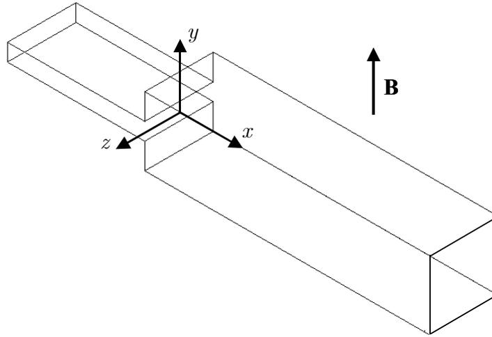
Figure 90: Geometry used in the experiments. The expansion ratio of the duct is 4 and the conductance parameter  $c$  is 0.03.
