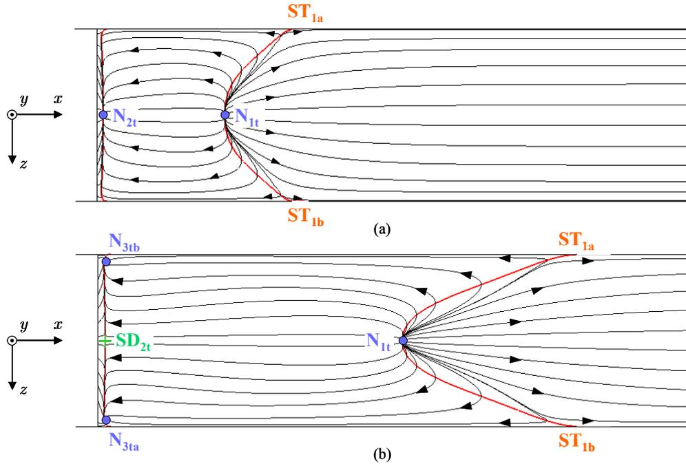
Figure 24: Limiting streamlines on the upper wall of the channel for the symmetric flows at  $Re = 10$  (a) and  $Re = 25$  (b). The topology close to the reattachment line remains the same while it changes near the expansion along the separation line.
