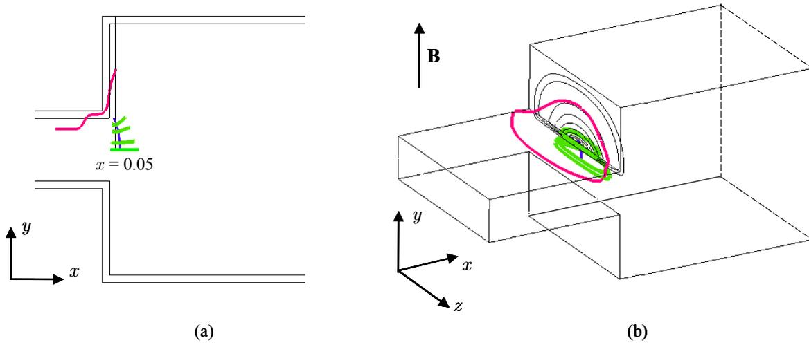
Figure 69: Current paths for  $Ha = 400$ ,  $N = 1600$  and  $c = 0.1$ . (a) The vertical line at  $x = 0.05$  indicates the plane on which limiting current streamlines are plotted. (b) Pseudo current streamlines are drawn in black.
