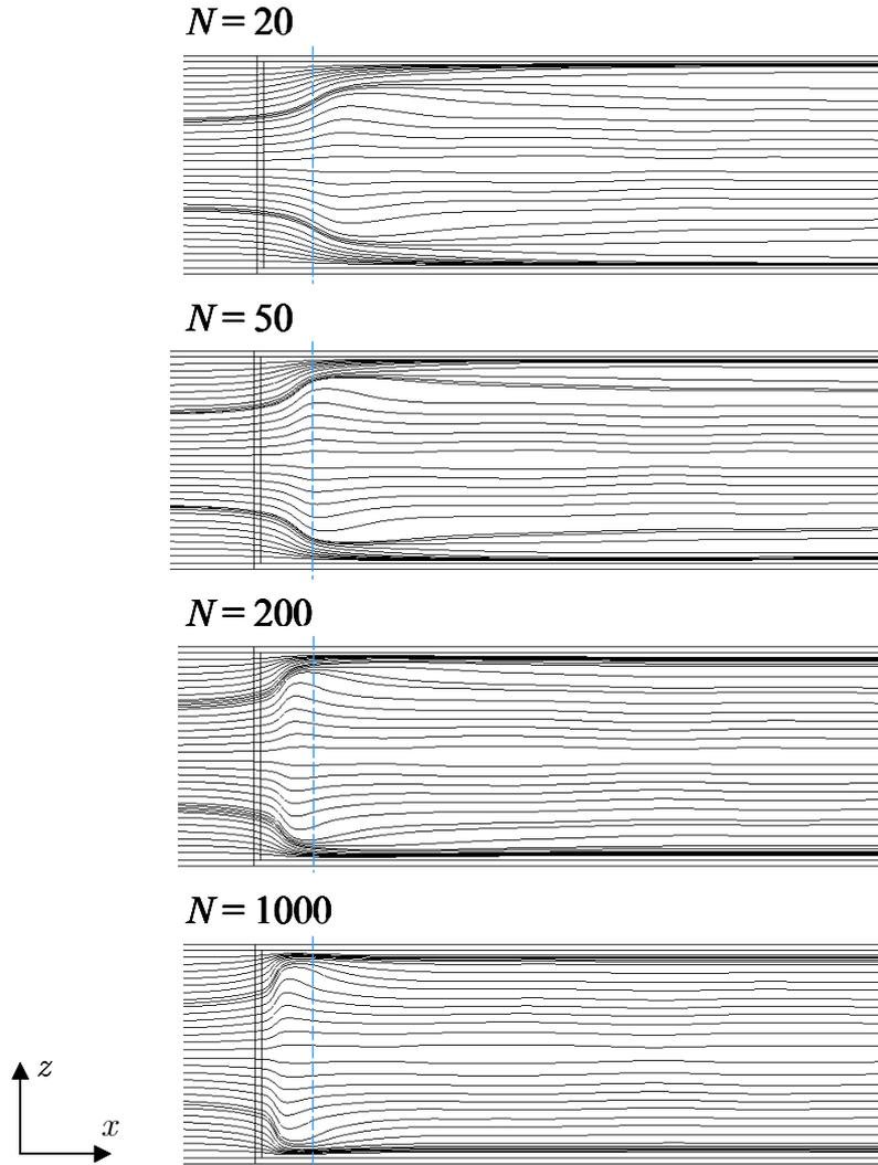
Figure 72: Velocity streamlines on the plane  $y = 0$  for the flow at  $Ha = 400$ ,  $c = 0.1$  and various interaction parameters  $N$  ( $Re = Ha^2/N$ ). The blue lines, located at  $x = 0.5$  are used as reference mark.
