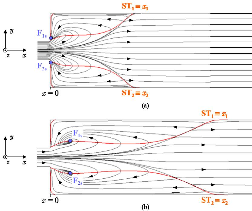
Figure 19: Limiting streamlines on the lateral wall of the duct for the flow at  $Re = 10$  (a) and  $Re = 20$  (b). The red lines indicate the locations where the  $u$ -velocity component is zero.  $ST$  designates the stagnation points and  $F_s$  the foci on the side wall.
