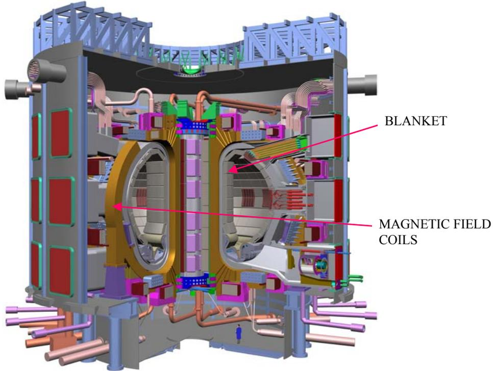
Figure 1: General view of the proposed international experimental fusion reactor (ITER).
