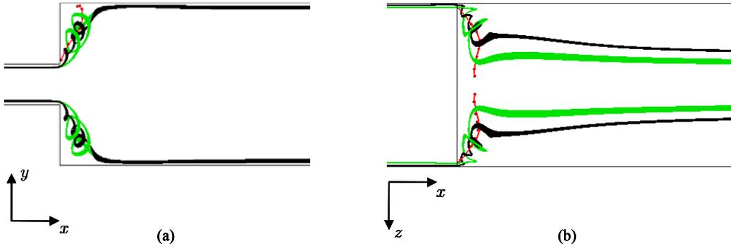
Figure 37: 3D streamlines for the flow at  $Ha = 30$ ,  $N = 9$  ( $Re = 100$ ) and  $c = 0.1$ . The lateral view shows the upward motion (a) and the top view the movement to the middle of the duct (b). The red line is the centre of the vortical structures.
