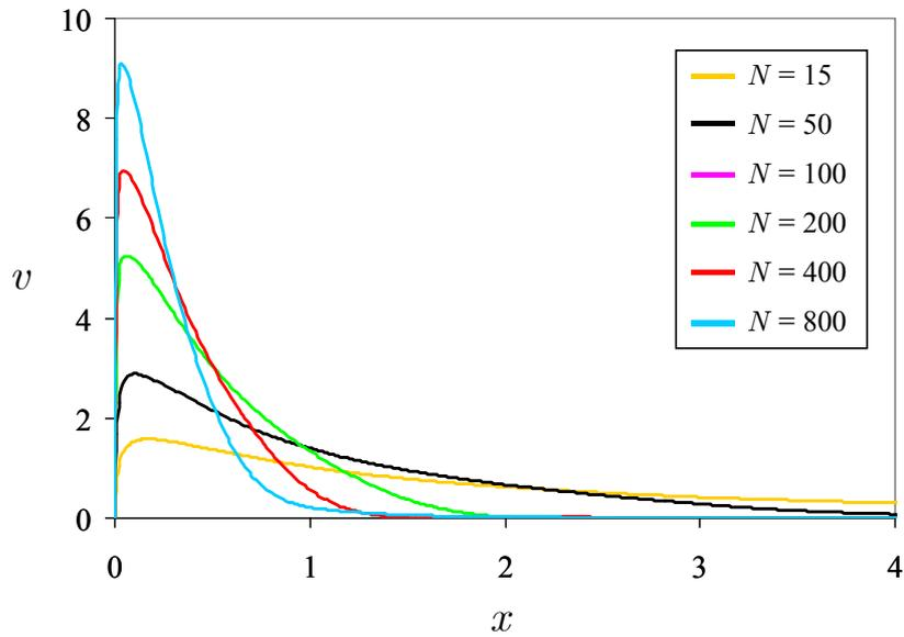
Figure 77: Vertical velocity plotted along the  $x$  direction near the internal edge of the expansion at  $y = 0.25$ , close to the side wall at  $z = 0.98$  for  $Ha = 400$  and various interaction parameters  $N$ .
