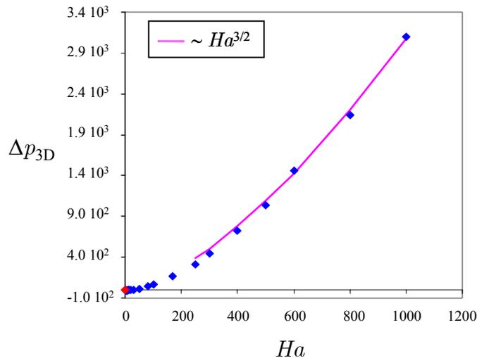
Figure 45: Pressure drop  $\Delta p_{3D}$  as a function of the Hartmann number. The continuous line is the best fit of the numerical results for high Hartmann numbers.
