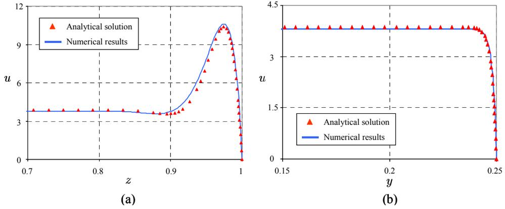
Figure 9: Calculated velocity profiles are compared with the analytical solution for  $c = 0.1$  and  $Ha = 500$ .
