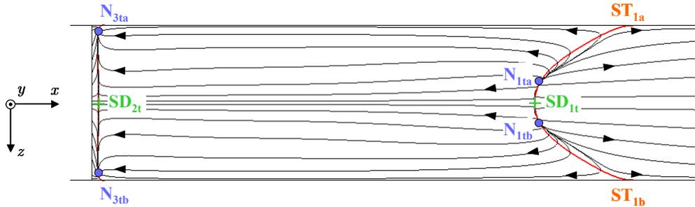
Figure 25: Limiting streamlines on the top of the duct for  $Re = 30$ . Downstream, along the reattachment line new topological features are present: two reattachment nodes acting as sources and a saddle point.
