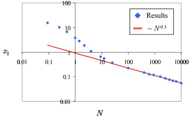
Figure 31: Reattachment length  $x_1$  at the side walls as a function of the interaction parameter  $N$  in logarithmic scale for  $Re = 100$ . The curve that fits well the results is proportional to  $N^{-0.3}$ .
