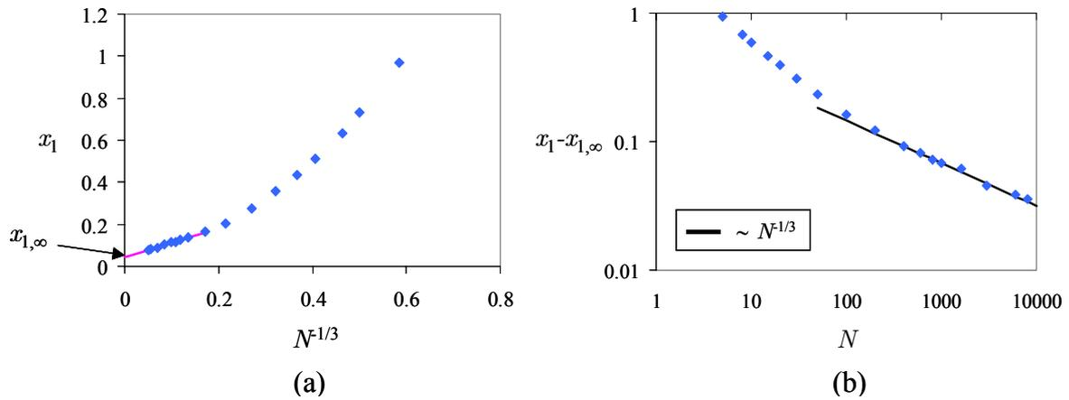
Figure 83: (a) Axial position of the point  $x_1$  on the side wall that bounds the back flow region, plotted as a function of  $N^{-1/3}$ .  $x_{1,\infty}$  is the value of the reattachment length in the inertialess limit ( $N \rightarrow \infty$ ). (b) Inertial part of the reattachment length versus  $N$ .
