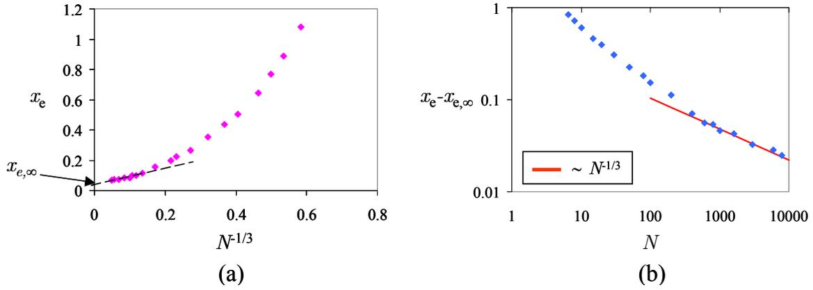
Figure 86: (a) Thickness of the internal layer as a function of  $N^{-1/3}$  for  $Ha = 400$ . (b) Thickness of the inertial part of the internal layer  $x_e - x_{e,\infty}$  plotted versus the interaction parameter  $N$  in logarithmic scale.
