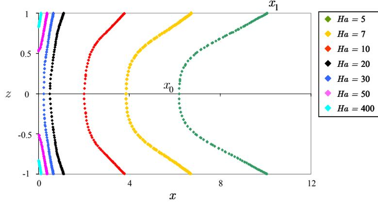
Figure 33: Lines along which the velocity component  $u$  vanishes, drawn on the Hartmann wall for various Hartmann numbers  $Ha$  and  $Re = 100$ .  $x_1$  and  $x_0$  are the reattachment points on the side wall and on the symmetry plane, respectively.
