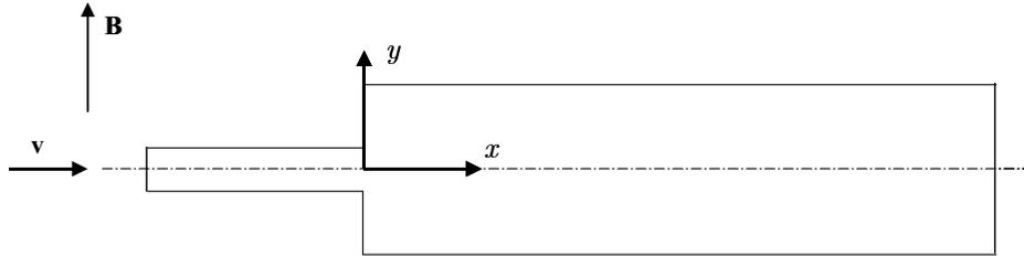
Figure 11: Sketch of the plane symmetric sudden expansion.
