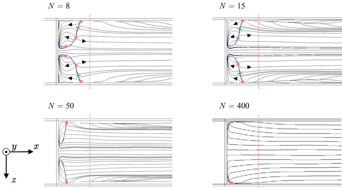
Figure 80: Limiting velocity streamlines plotted on the Hartmann walls for  $Ha = 400$  and four different interaction parameters  $N$ . The red dots indicate critical points acting as sources, the green crosses are saddle points and the circles present for  $N = 8$  are foci. The dashed lines are located at  $x = 1$  as reference mark.
