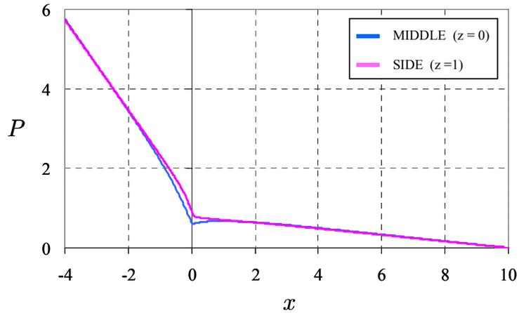
Figure 50: Pressure variation along the centerline of the duct ( $z = 0$ ) and at the side wall ( $z = 1$ ) for  $Ha = 700$  and  $N = 4900$ . In the figure  $P = p/N$ , where  $p$  is the pressure in the hydrodynamic scale.
