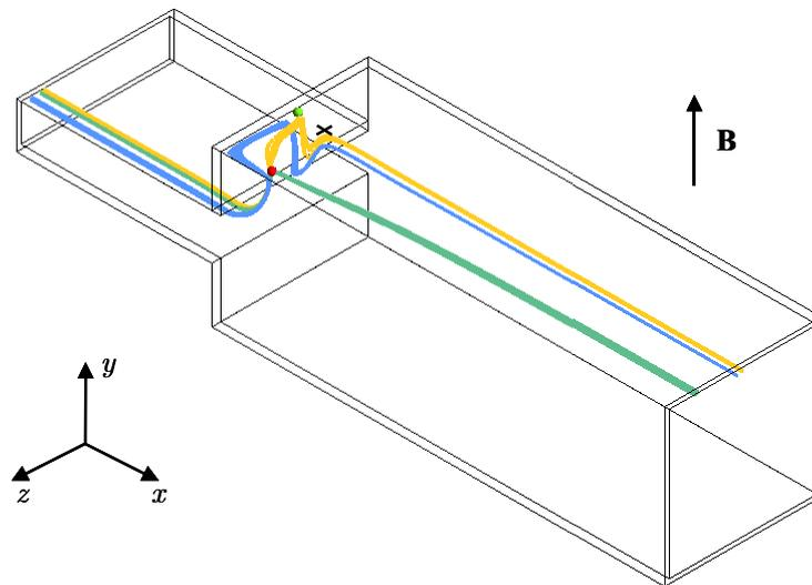
Figure 39: Flow at  $Ha = 30$ ,  $N = 9$  and  $c = 0.1$ . The streamlines show the meaning of the critical points characterizing the flow topology on the Hartmann wall. The red point is the source, the green one is the sink and the cross is the saddle point.
