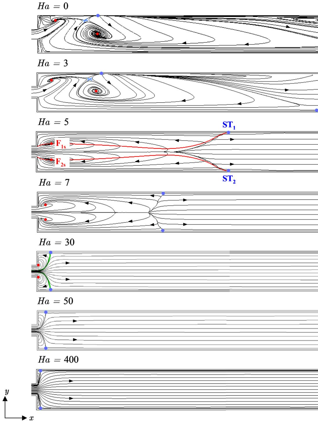
Figure 29: Limiting velocity streamlines on the side wall parallel to  $\mathbf{B}$  for  $c = 0.1$ ,  $Re = 100$  and various Hartmann numbers  $Ha$ . The red points are the foci, traces on the side wall of vortical structures, and the blue dots on the Hartmann walls are the reattachment points. Along the red line, plotted for  $Ha = 5$ , the axial velocity is zero. The green line drawn for  $Ha = 30$  indicates the reattachment line.
