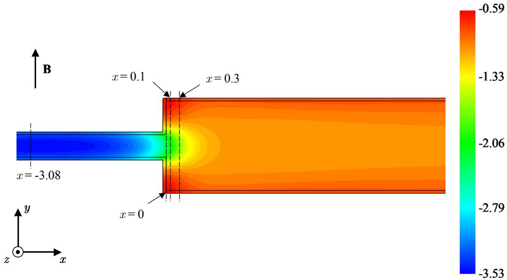
Figure 92: Contour plots of the calculated electric potential on the side wall of the duct for the flow at  $Ha = 500$ ,  $N = 50$  and  $c = 0.03$ . The numerical results are compared with the experiments along the dashed lines (Figs.93 and 94).
