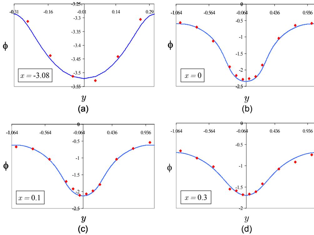
Figure 93: Electric potential on the side wall plotted along field lines at different axial locations. The symbols are the experimental data and the lines the numerical results for the flow at  $Ha = 500$ ,  $N = 50$  and  $c = 0.03$ .
