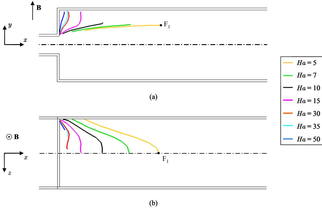
Figure 40: Vortex core lines for several Hartmann numbers and  $Re = 100$ .  $F_1$  is the trace of the vortex core line on the symmetry plane  $z = 0$ .
