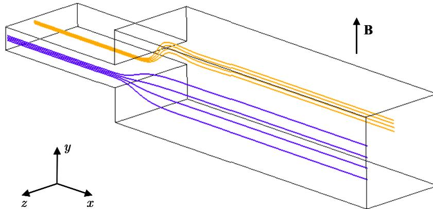
Figure 35: Flow at  $Ha = 30$ ,  $N = 9$  ( $Re = 100$ ) and  $c = 0.1$ . Flow from the upstream core enters the downstream core (orange path) and flow in the side layer, far from Hartmann walls, stays in this layers moving downstream (blu lines).
