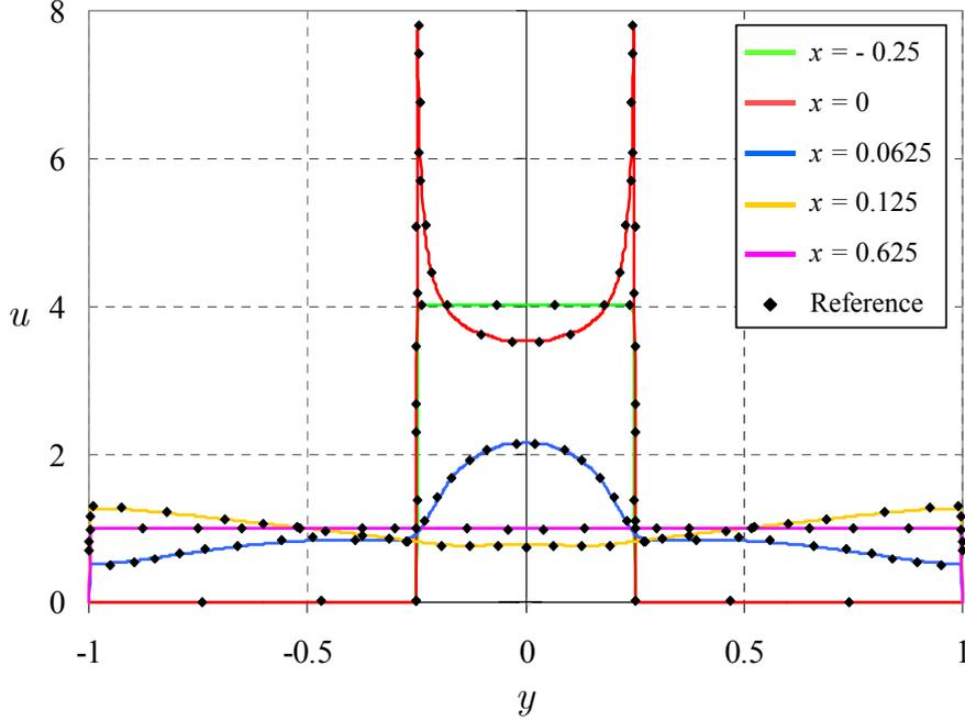
Figure 13: Velocity component  $u$  versus the vertical direction  $y$ , parallel to the magnetic field, at different axial positions. The results are calculated using *grid D*. The symbols correspond to the solution reported by Aleksandrova et al. (2003).
