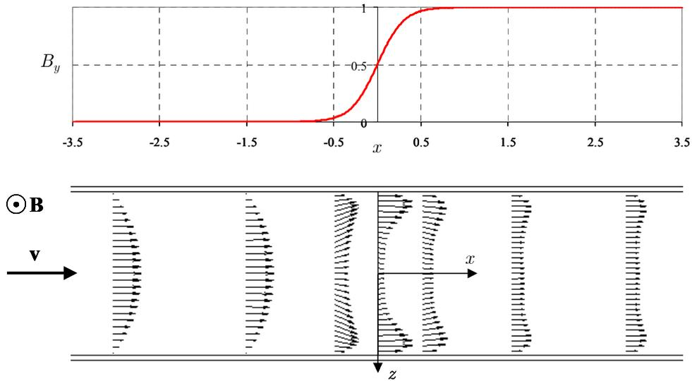
Figure 18: The upper curve is the imposed magnetic field. The vector plots illustrate the redistribution of the velocity in the plane  $y = 0$  perpendicular to the B-field for the flow at  $Ha = 50$ ,  $N = 1000$ ,  $c = 0.1$ .
