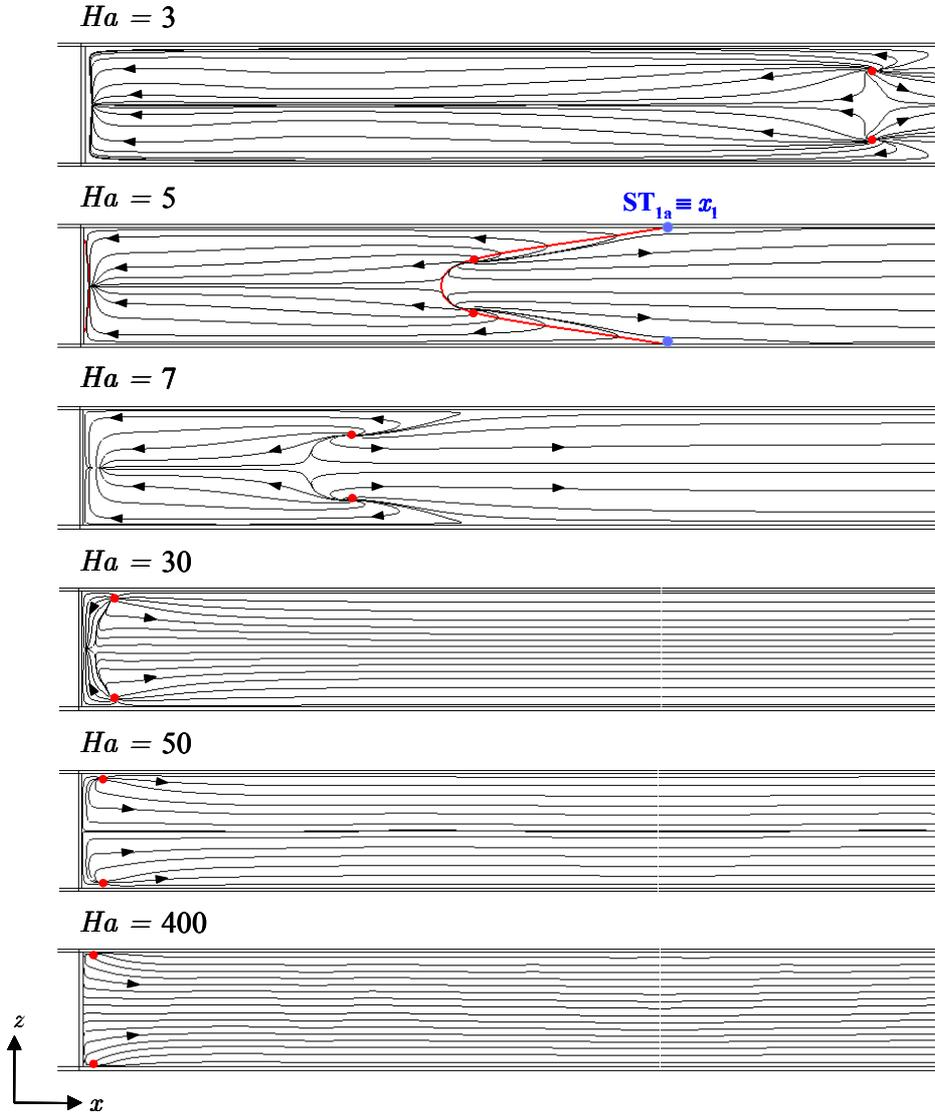
Figure 32: Limiting streamlines on the wall perpendicular to the magnetic field for various Hartmann numbers  $Ha$  and  $Re = 100$ . The red points are the nodes that behave as sources of streamlines.
