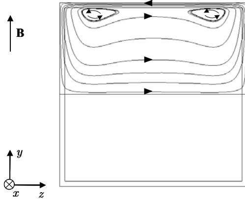
Figure 63: For the flow at  $Ha = 50$ ,  $N = 25$  and  $c = 0.1$  the current distribution in a cross-sectional plane ( $x = 2$ ), behind the area of strong 3D phenomena, shows two small local loops inside larger paths.
