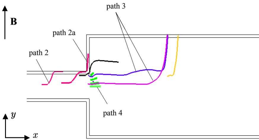
Figure 65: Projection of current streamlines on a  $xy$  plane for the flow at  $Ha = 400$ ,  $N = 1600$  and  $c = 0.1$ .
