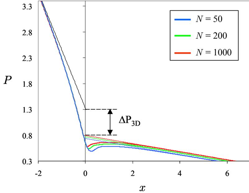
Figure 88: Pressure distribution along the axis of the duct for  $Ha = 400$  and three interaction parameters  $N$ . The straight lines indicate the fully developed pressure gradients in the small and in the large channel. The additional pressure drop due to 3D MHD effects is indicated by  $\Delta P_{3D}$  for  $N = 1000$ . The quantity  $P$  is given by  $p/N$  where  $p$  is the pressure in the hydrodynamic scale.
