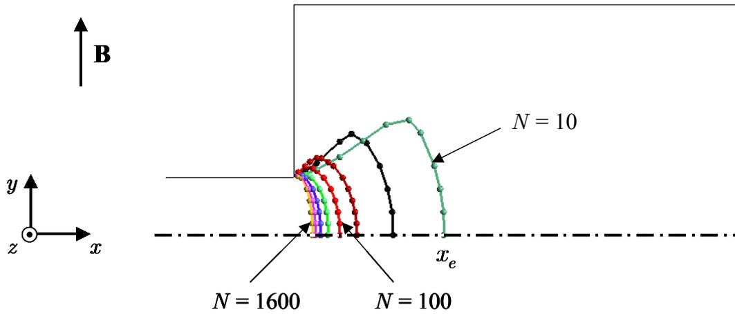
Figure 85: Centerlines of the current tubes that form in the core region of the duct for  $Ha = 400$ .  $x_e$  is the centre of the current loop on the plane  $y = 0$  and it is used as a measure for the thickness of the internal layer.
