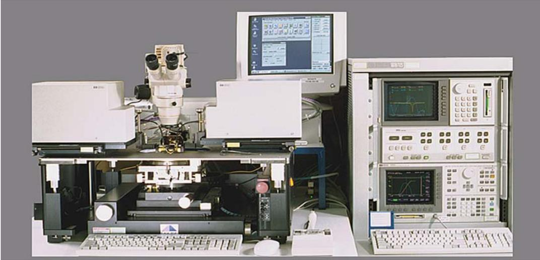
Figure 4.2: Photograph of S-parameter measurement system HP 8510XF.
