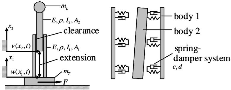
Fig. 1: a) System model, b) Contact formulation.
