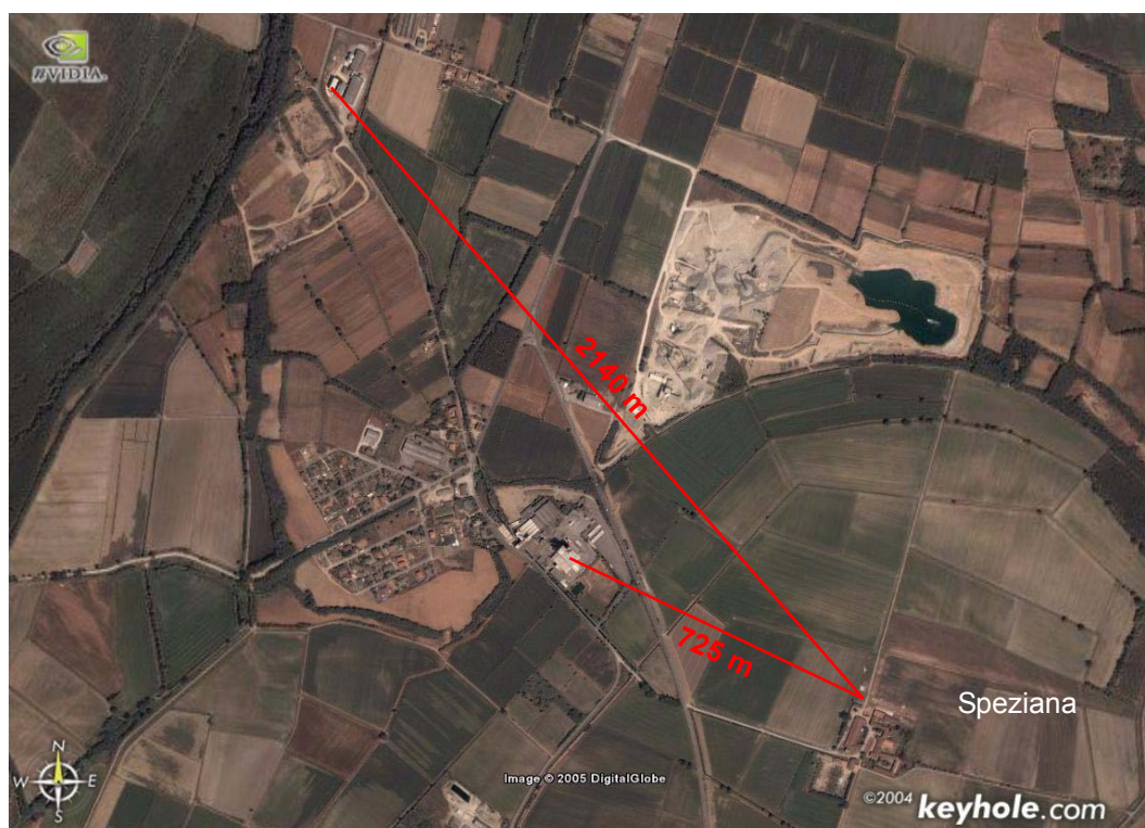
Figure 4.13: Agricultural surroundings of the farm 'Speziana' at Spessa including the DOAS light paths and their path lengths (one way).
