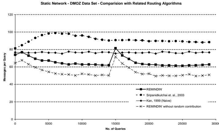
Figure 7.9.: Static Network: Comparison of Query Routing Algorithms: Messages per Query
