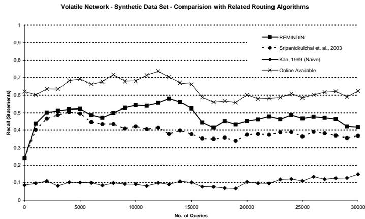
Figure 7.16.: Volatile Network: Comparison of Query Routing Algorithms – Conjunctive Queries – Synthetic Data Set: Recall
