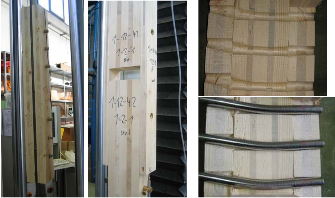
Fig. 10: Test-setup for connections 1-24-2S_1.1 and 1-12-42_1.2, opened connection 1-20-22_1.2.2 (right)
