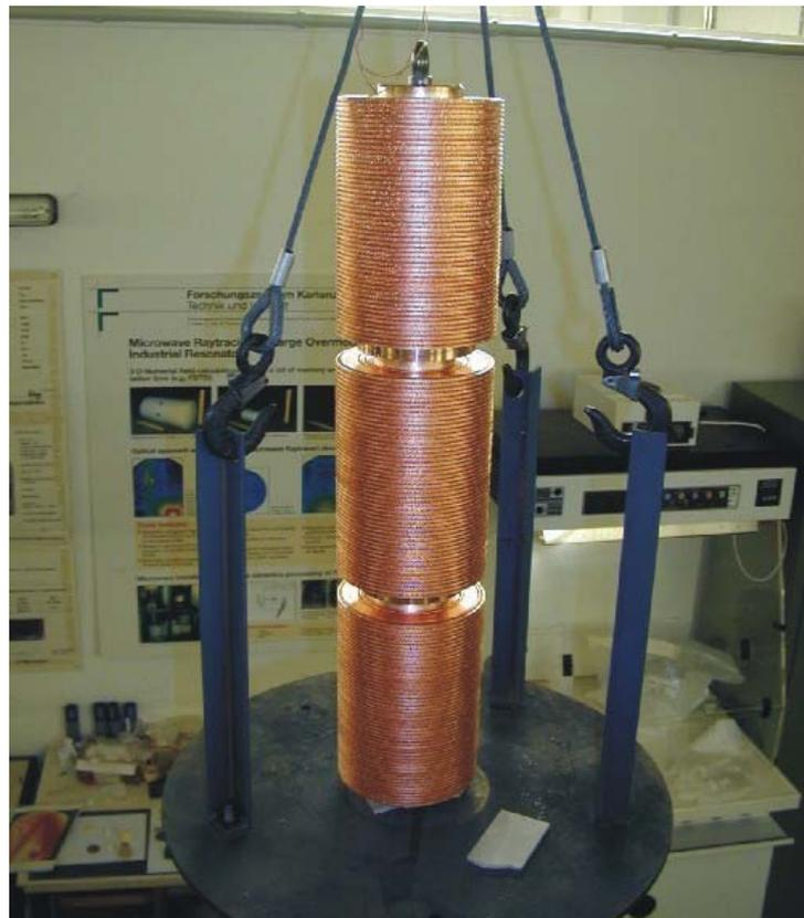
Figure 8.15 Photograph of the conventional heat exchanger of the 70 kA HTS current lead [63]
