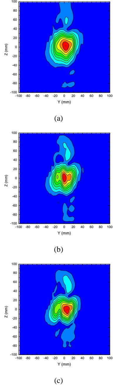
Fig. 3. Calculated field distribution on the last mirror. Normalized field contours are shown in linear scale with 0.1 increments from the peak: (a)  $TE_{17,6}$  mode, (b)  $TE_{20,7}$  mode, (c)  $TE_{22,8}$  mode.
