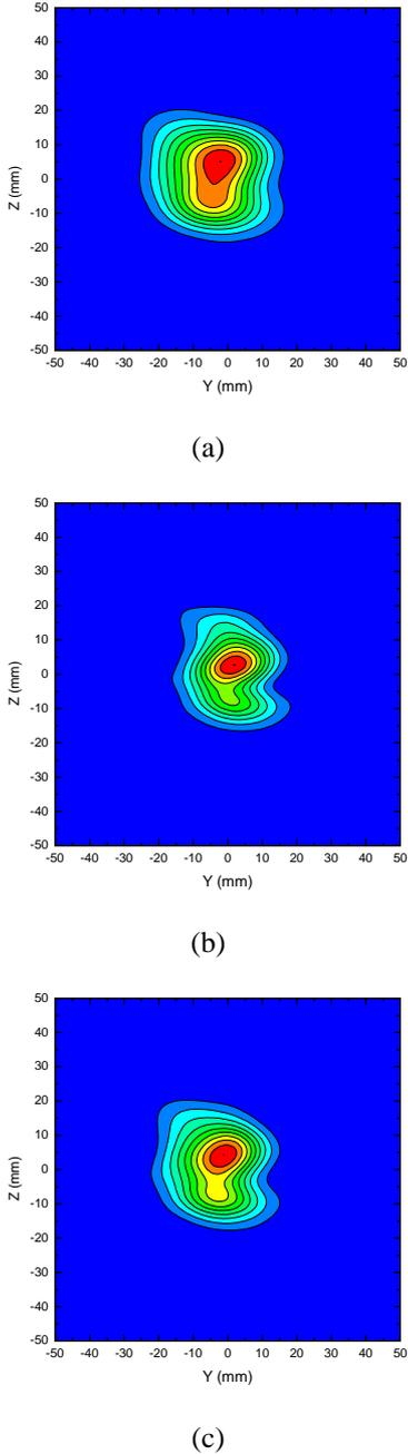
Fig. 4. Calculated power distribution at the middle position of the Brewster window. Normalized power contours are shown in linear scale with 0.1 increments from the peak: (a) TE<sub>17,6</sub> mode, (b) TE<sub>20,7</sub> mode, (c) TE<sub>22,8</sub> mode.
