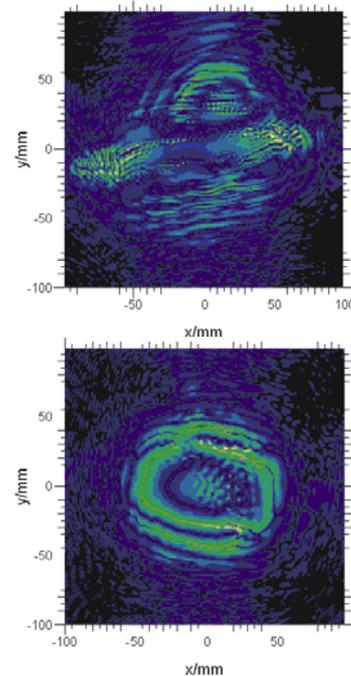
Fig. 1. Mirror surface of existing adapted phase-correcting mirror2 (upper) and phase-correcting mirror3 (lower).
