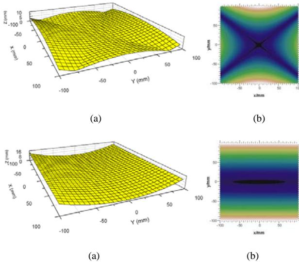
Fig. 2. Calculated mirror surface (a) and surface contour (b) of elliptical mirror 2 (upper) and elliptical mirror 3 (lower).
