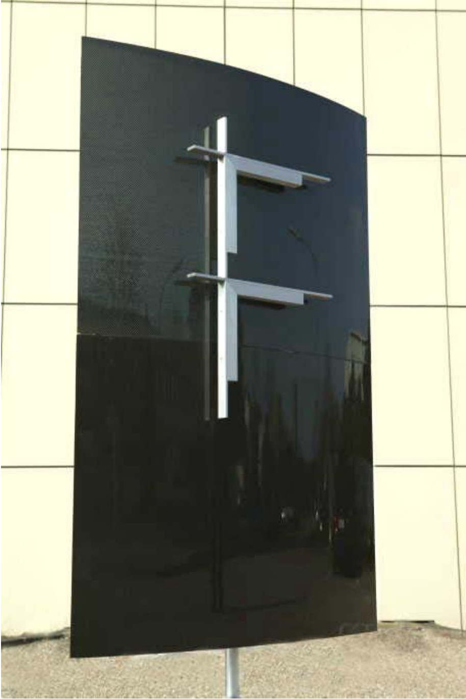
Figure 5.21 Photograph of a curved CFRP plate (1.26 m x 1.95 m ) processed in the HEPHAISTOS-CA2 oven
