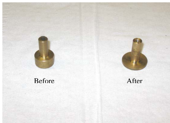
Figure 5.2 Photograph of the transition antenna before and after the optimization
