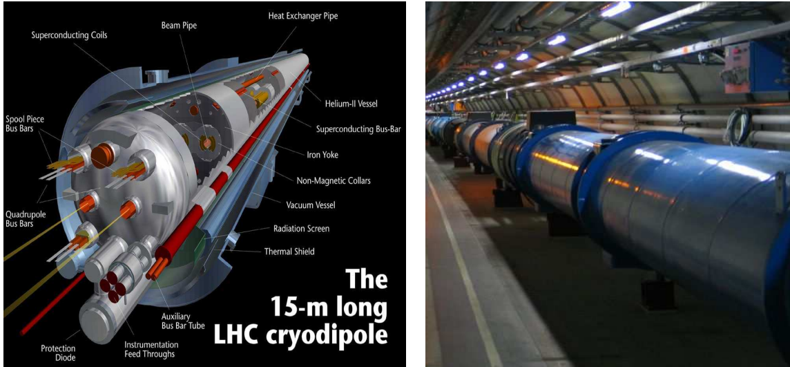
Figure 1.2: On the left: Schematic view of a LHC dipole magnet. On the right: the LHC tunnel with the installed magnets.
