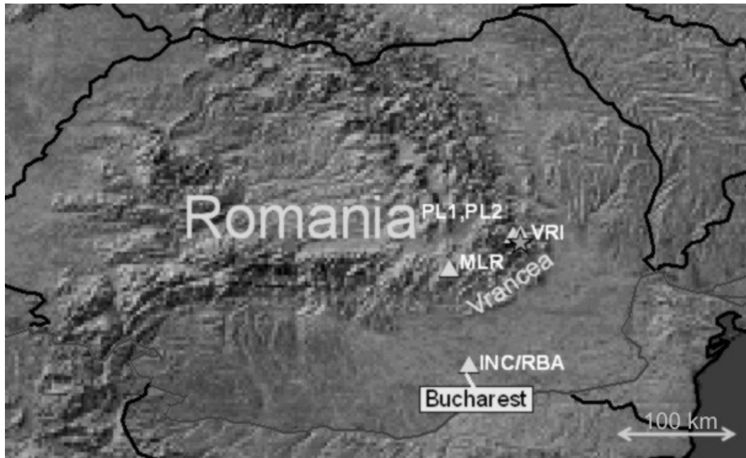
Figure 5.1: Distributions of accelerometers used for the Romanian earthquake early warning system and additional stations used for the definition of scaling relations.
