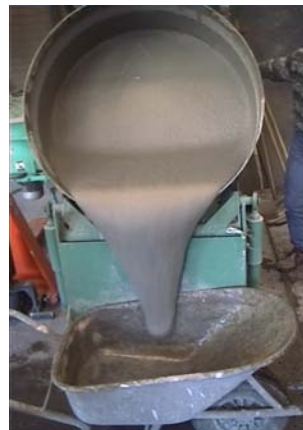
Fig. 18: Self-compacting fibre concrete after production
