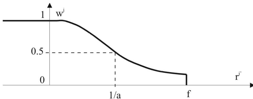
**Figure 4.3:** Parameters of the weight function. (Where  $w$  is the weight,  $a$  is the half weight filter value and  $f$  is the maximum filter value, where the weight is higher than 0.)
