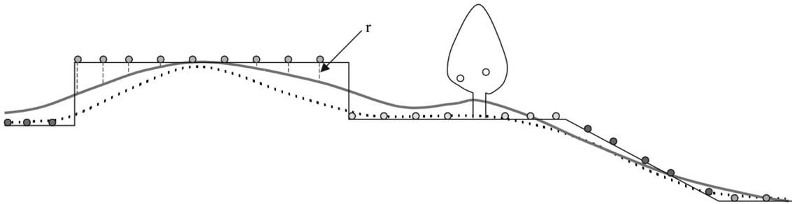
**Figure 4.2:** Segment based robust interpolation. The continuous line presents a trend surface in an early iteration, while dotted in a latter one. Points in the same greyscale belong to the same segment. Residuals to the trend surface are also shown at one segment.
