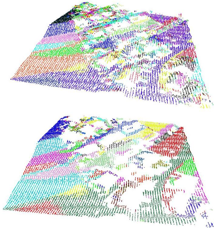
**Figure 7.1:** Segmented and filtered sample. On the top, the result of segmentation is presented. At the bottom, the resulted ground segments can be seen.
