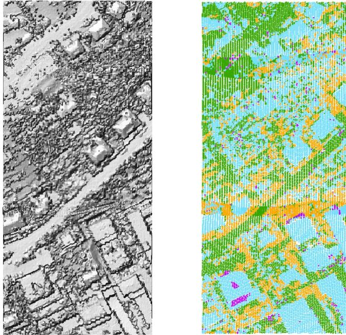
**Figure 7.2:** Sample 11. (Green - ground points, light blue - object points, orange - type II errors, purple - type I errors)
