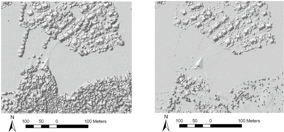
**Figure 2.6:** First pulse nDSM on the left side and last pulse nDSM on the right. It does not contain the influence of the topography (compare to 2.4). The complete vegetation can be observed on the first pulse nDSM, but only the partial vegetation on the last pulse nDSM.
