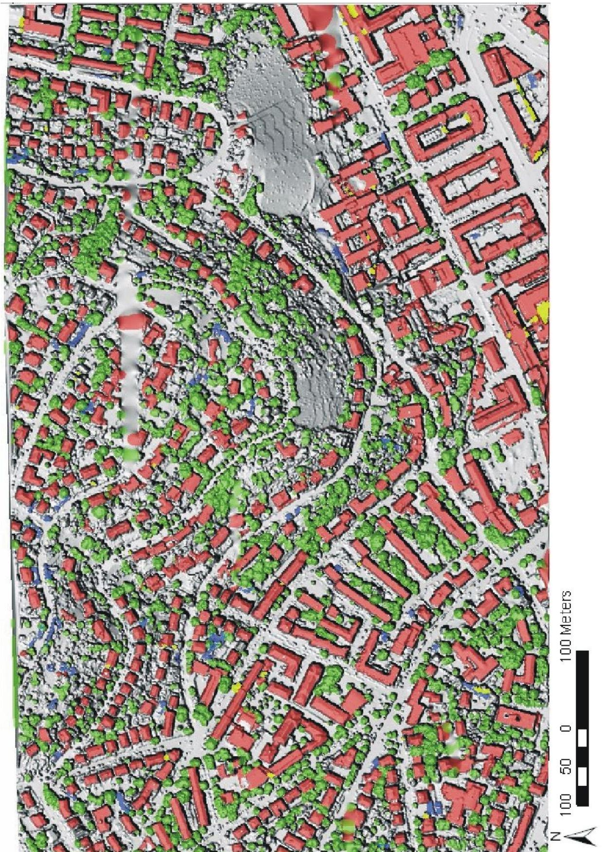
**Figure 7.23:** Classification result 'Stuttgart' test site. (Red - buildings, green - vegetation, yellow - misclassified vegetation, blue - misclassified buildings)
