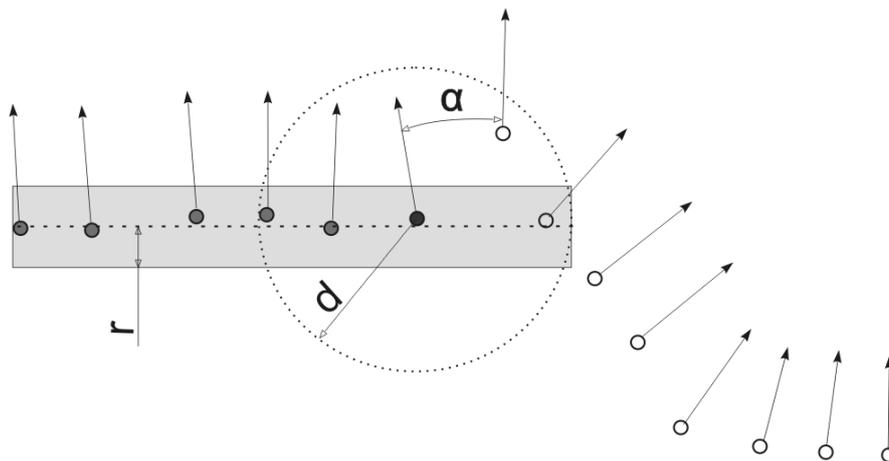
**Figure 5.2:** Parameters of the segmentation (gray points- accepted points, black point- actual point, white points- not (yet) accepted, dashed line- adjusting plane, arrows- normal vectors). The gray area represents the distance criterion of the point and the adjusting plane.
