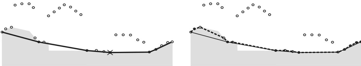
**Figure 4.1:** Convex concave hull approach. On the left: convex hull (line) is fitted on the data. On the right: convex hull densification by concave triangle nodes (dashed lines) [Steinle, 2005]
