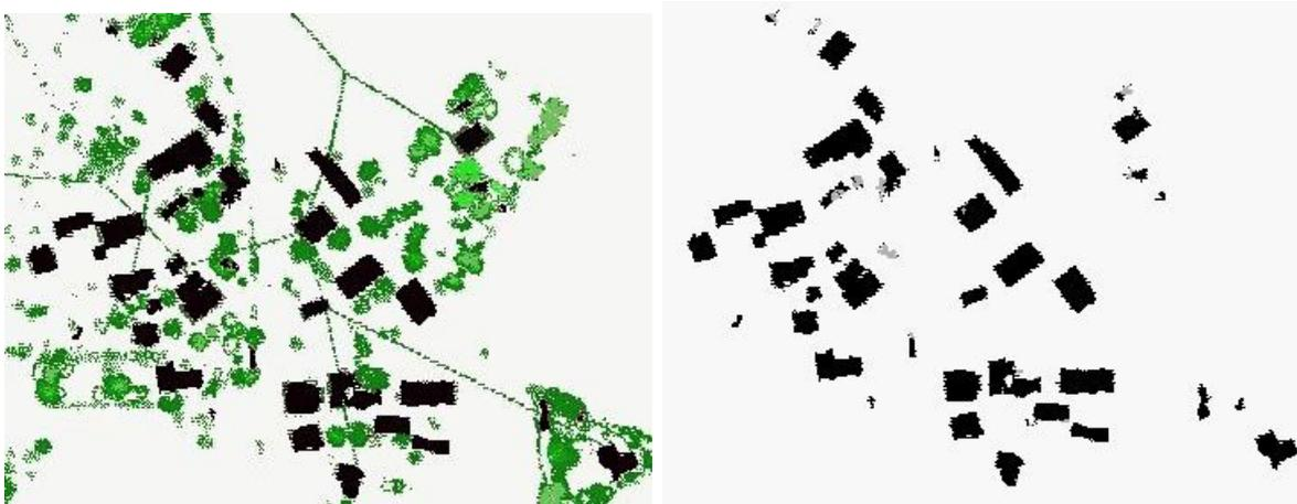
**Figure 5.5:** The effect of considering the first and last pulse differences. On the left, vegetation (green), power lines and buildings are presented. On the right, segmented buildings by first and last pulse differences (black) and original segments (grey) can be seen. Vegetation over the roof causes segmentation errors.
