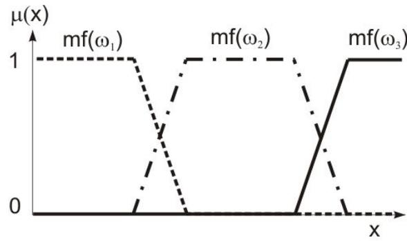
**Figure 6.11:** Membership functions of three classes ( $\omega_j$ ) for a feature
