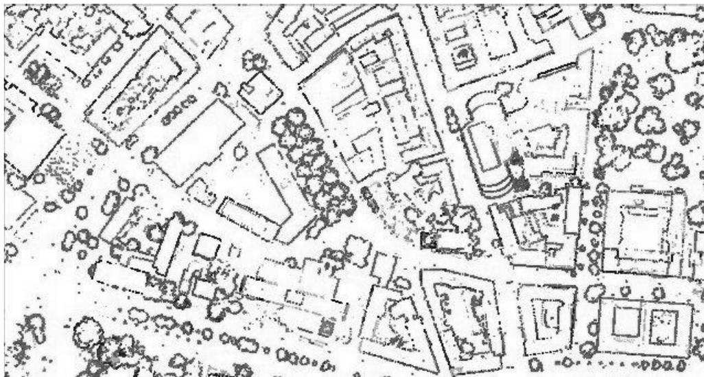
**Figure 6.3:** Differences between first and last echo (Schnadt, 2004). Data acquisition was carried out in summer and first and last pulse differences are calculated by every single measurement. Consequently these differences at the border of trees are significantly higher than inside.
