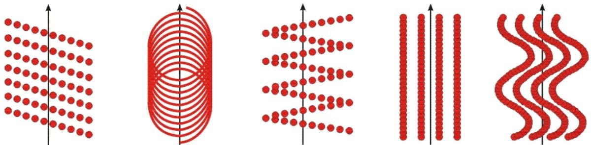
**Figure 2.2:** Footprints of scanning systems (rotating polygon, nutating mirror, rotating mirror, fiber, fiber with swing mode)(Steinle, 2005)
