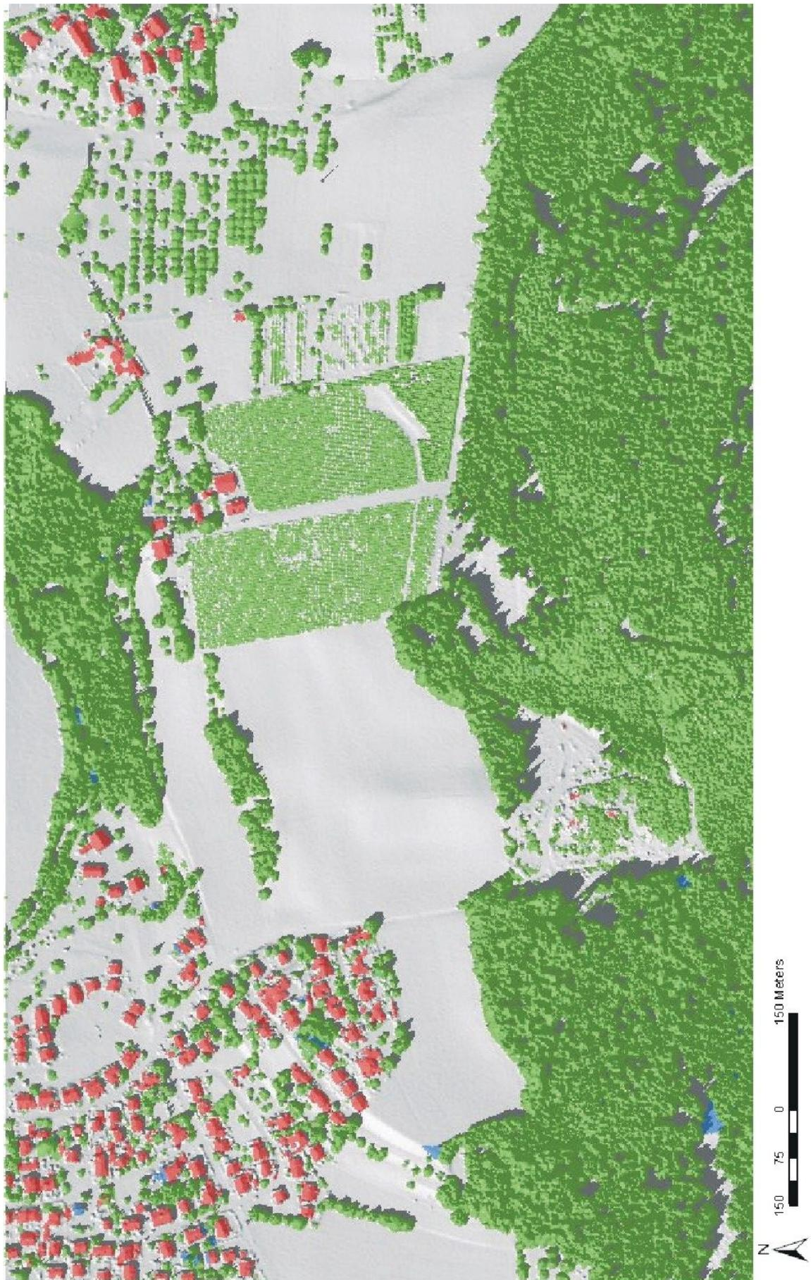
**Figure 7.22:** Classification result of 'Salem' test site. (Red-buildings, green-vegetation, blue-terrain objects and gray-terrain)
