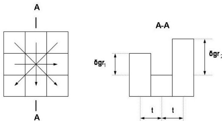
**Figure 6.6:** Local curvature computation. A 3x3 raster kernel can be seen. Arrows show the four directions of the gradient calculation.
