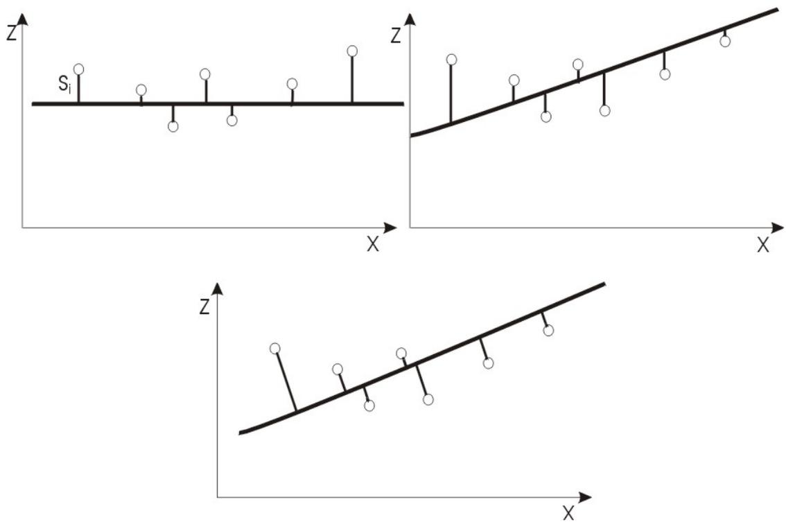
**Figure 6.4:** Computation of root mean square errors. Measurements are represented by circles, the trend surface and residuals are represented by lines. Standard deviation over a horizontal plane is shown on the left, 2.5 D solution over a tilted plane on the right, and 3 D solution at the bottom.
