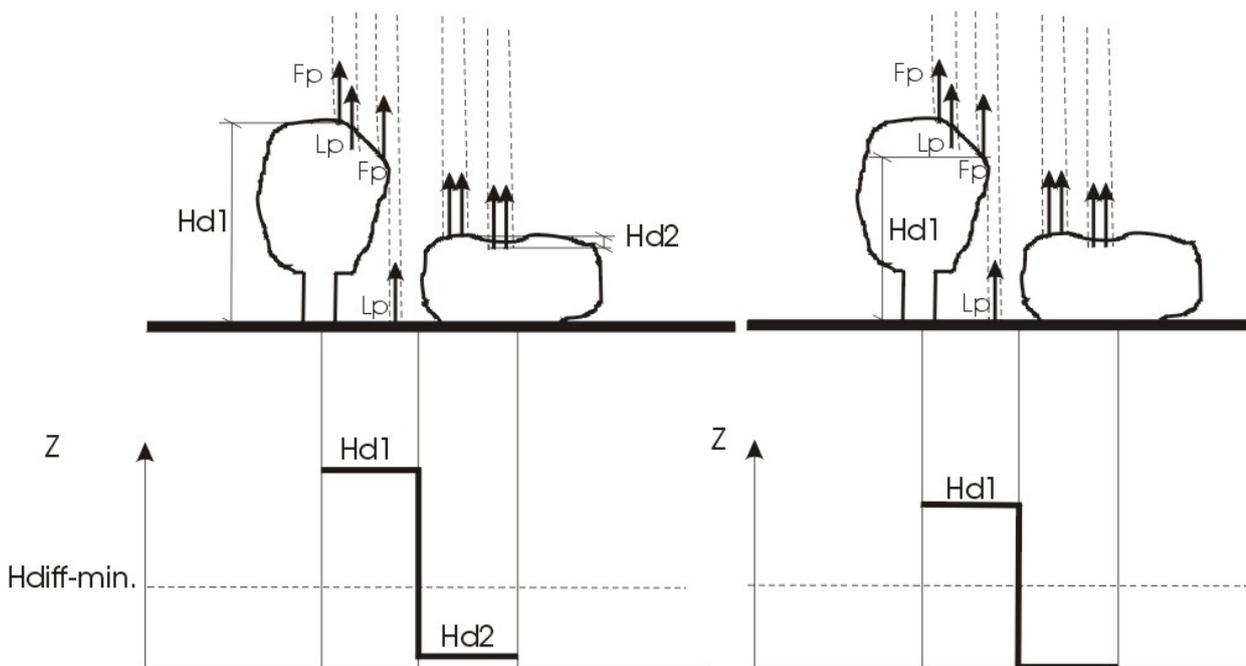
**Figure 6.1:** Calculation methods of first and last pulse differences. 2-2 raster elements are presented in each figure. On the bottom, the calculated values can be seen. On the left side, differences are calculated within a raster, therefore the rasterisation has an effect on the values. On the right, values represent the real differences between the corresponding first and last pulses.
