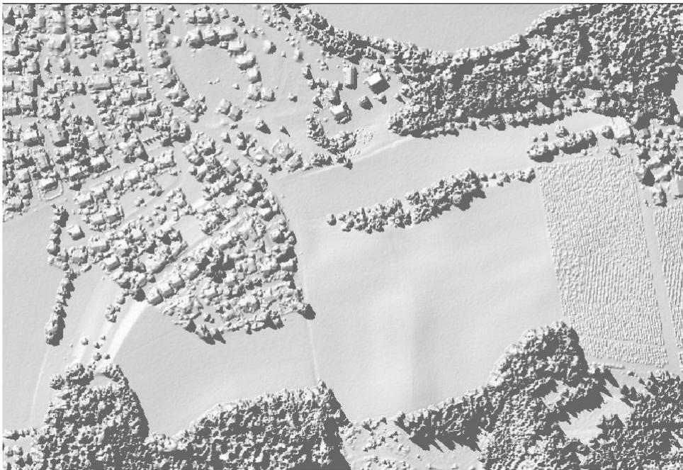
**Figure 7.20:** First pulse DSM of the 'Salem' dataset.
