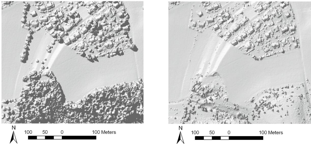
**Figure 2.4:** First pulse DSM on the left and last pulse DSM on the right.
