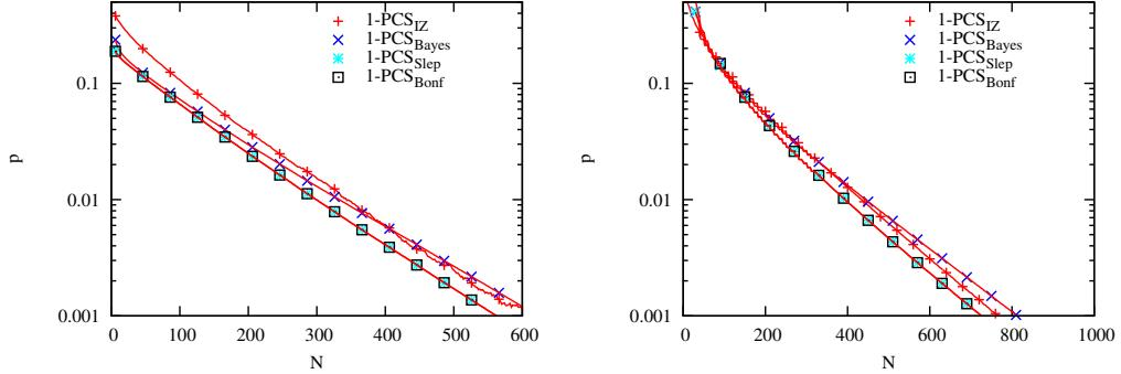
Figure 2.2: Different measures and approximations for correct selection (Equal samples for  $k = 2$  systems with a difference of  $\delta = 0.25$  (left) and  $k = 10$  with a difference  $\delta = 0.5$  of neighboring systems (right). The variances of all systems are equal).
