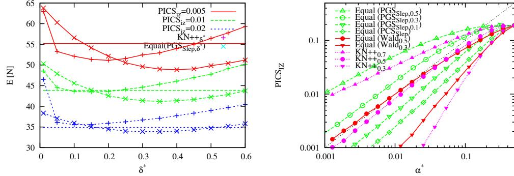
Figure 2.6: Influence of  $\delta^*$  on the mean number of samples to obtain a desired  $\text{PICS}_{\text{IZ}}$ , for  $\mathcal{KN}++$  and  $\text{Equal}(\text{PGS}_{\text{Slep},\delta^*})$  (SC,  $k = 2$ ,  $\delta = 0.5$ ,  $\rho = 1$ ).
