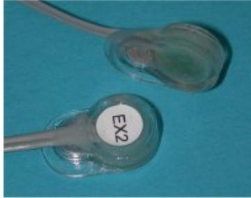
**Figure 4.15.** The Flat-Type Active Electrodes for Multi-channel ECG *ActiveTwo* System. Figure is adopted from [131]
