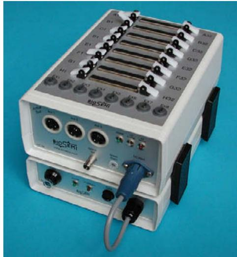
**Figure 4.17.** Multi-channel ECG *ActiveTwo* AD-box with battery. Figure is adopted from [131]
