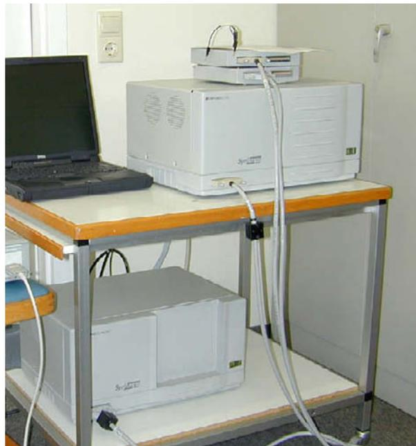
Figure 4.13. Two *SynAmps* main units and two *headboxes* placed on one of the main unit
