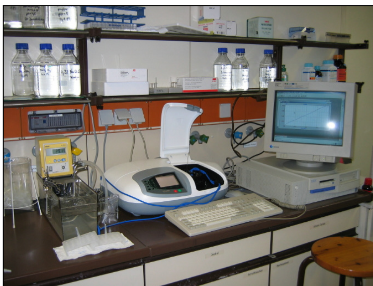
Figure 10: Device used for spectrophotometric assay for the direct determination of micro magnetic particle immobilised lipase activity.
