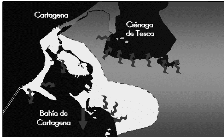
Fig. 98: Existing wastewater / drainage situation, where raw sewage flows in open canals or sewers to either the Bahía de Cartagena (40%) or the Ciénaga de Tesca (60%) causing considerable environmental and public health impacts (courtesy of M. Libhaber, World Bank)
