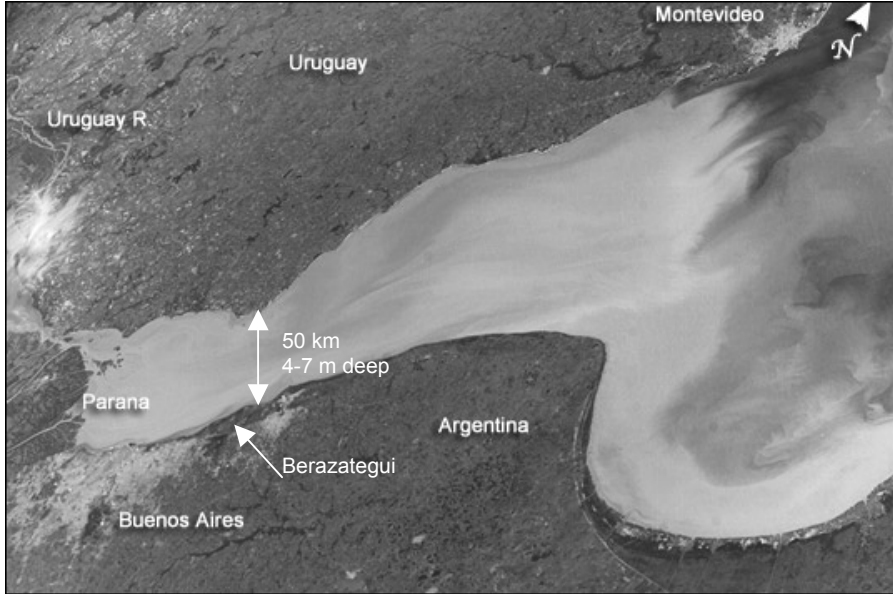
Fig. 50: Top view of the Rio de la Plata delta showing the location of the Berazategui outfall and the ambient characteristics at its location (source: Nasa, 2005)
