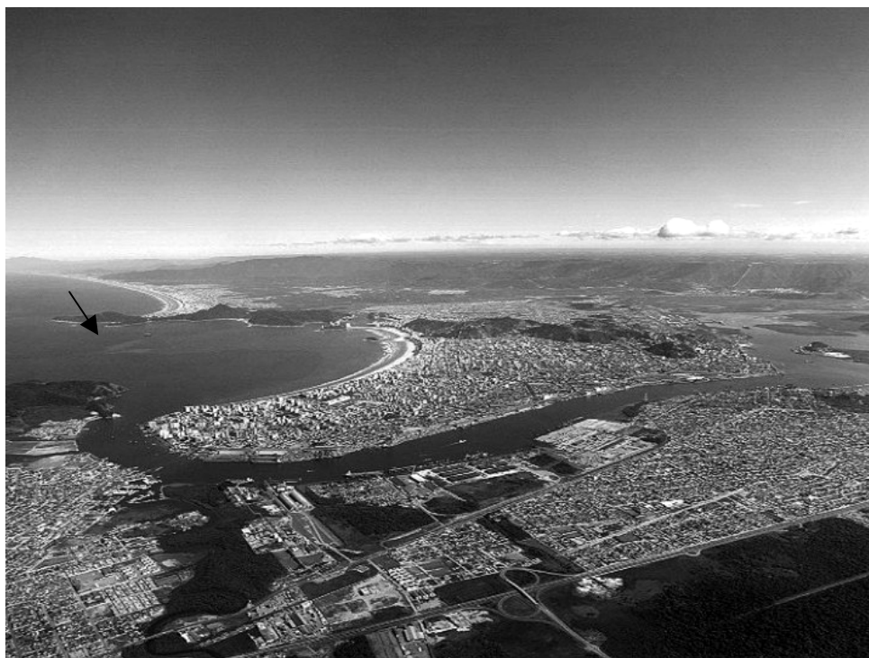
Fig. 2: Aerial photograph of Santos Bay, Brazil showing Santos city (approx. 500,000 inhabitants) and Santos harbor (along the river). Visual contours of the waste plume (arrow) from the Santos outfall, 4 km offshore, show a plume impact with the city's most frequented beaches (courtesy of municipality of Praia Grande, Brazil).
