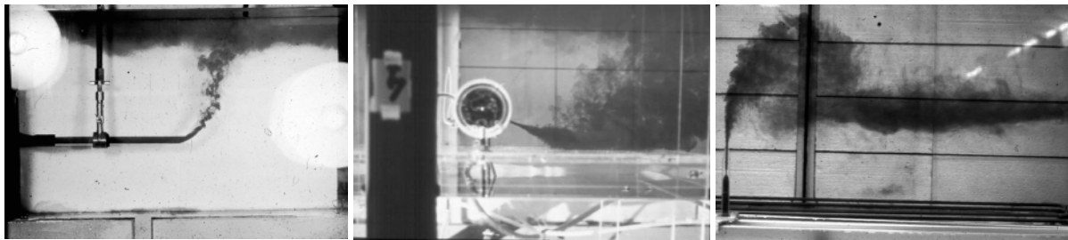
Fig. 65: Pictures of laboratory experiments showing boundary interactions with the surface, the bottom and the pycnocline (courtesy of G.H. Jirka, L. Fan, Keck Lab, CIT)
