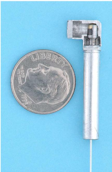
a) ISL cooling line with connection elbow
