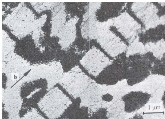
Fig. 2-7 TEM image of dislocation structures (PSBs) in a fatigued Cu crystal [Mughrabi1979].
