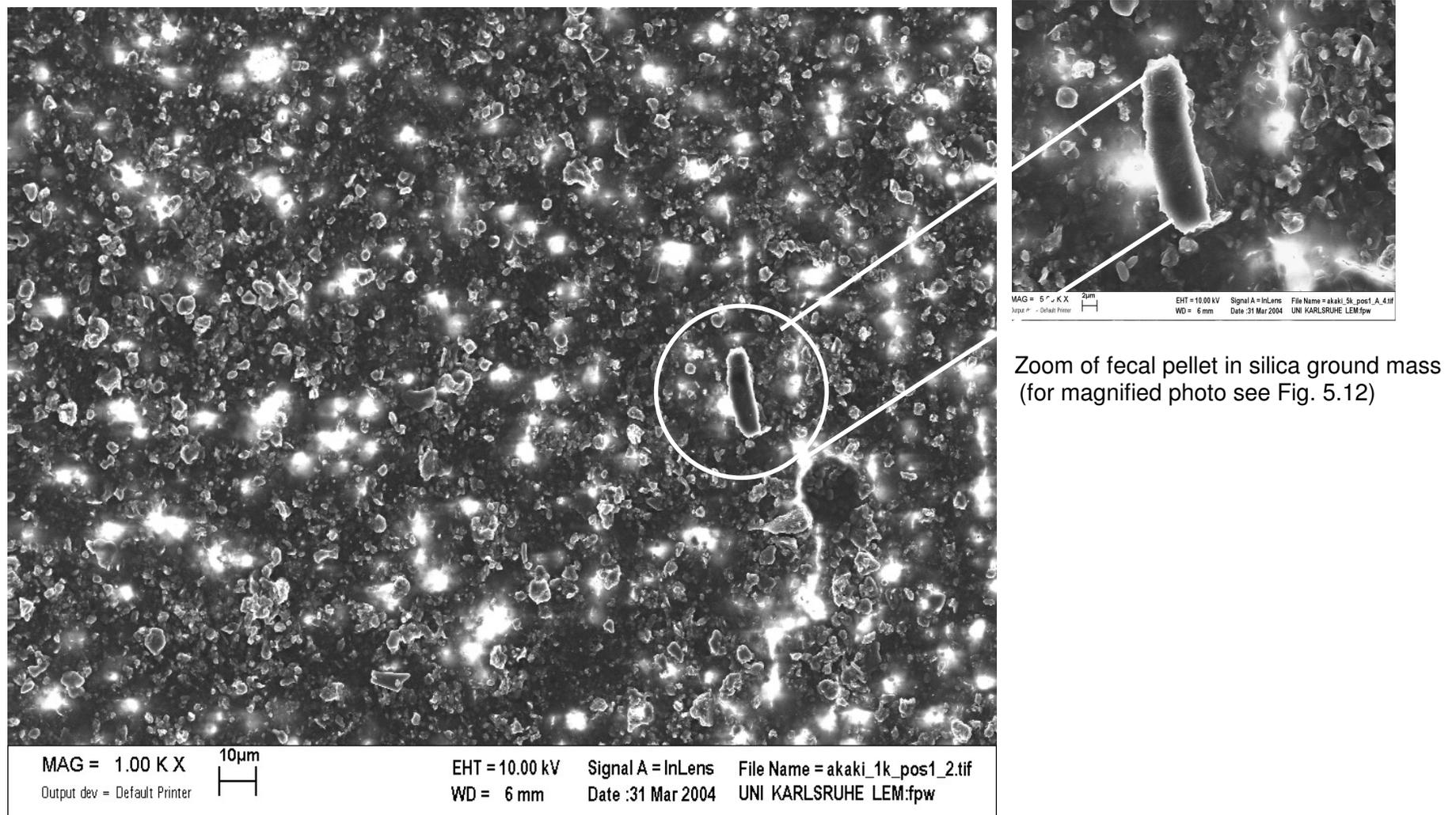
Fig. 5.11. SEM photo of the matrix of SPM taken from the Little Akaki River at sample site EI18 (ELICO).
