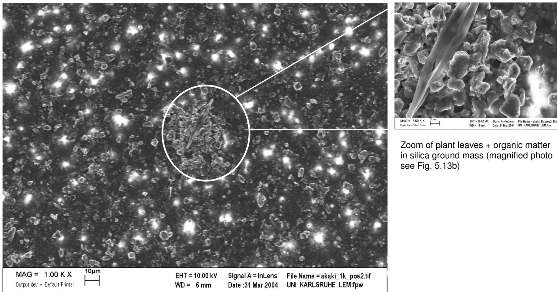
Fig. 5.13a. SEM photo of the matrix of SPM taken from the Little Akaki River at sample site E118 (ELICO). Elongated plant leaves represent organic matter.
