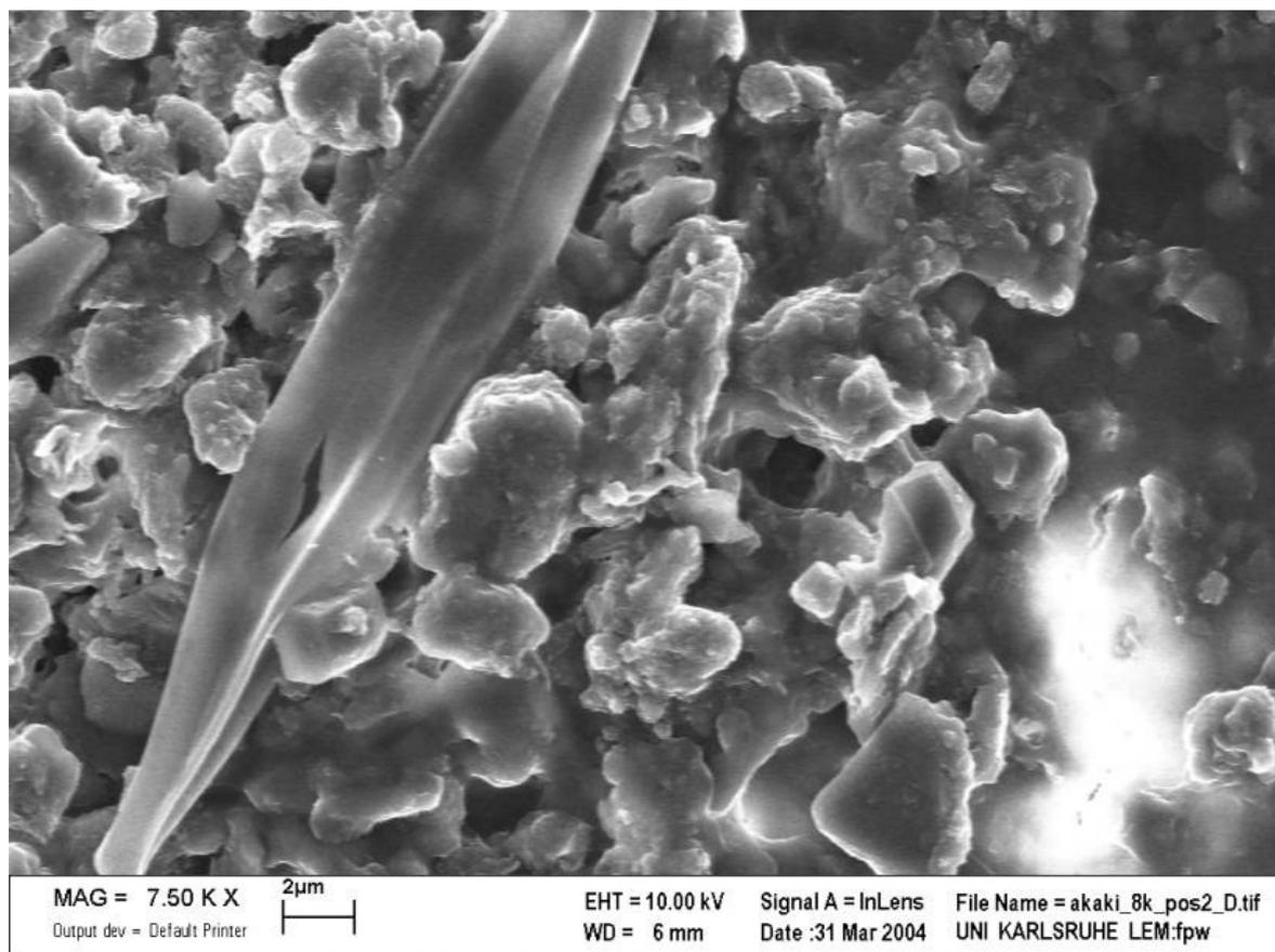
Fig. 5.13b. SEM photo of SPM taken from the Little Akaki River at sample site EI18 (ELICO). Elongated plant leaves and other remains of organic matter represent organic fraction.
