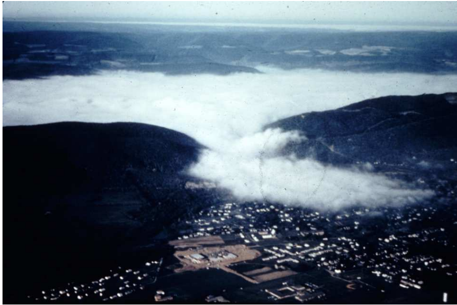
Figure 1.2: An example of stratified exchange flow in the atmosphere: fog sea in a Rinevalley, flowing into another valley due to temperature differences.
