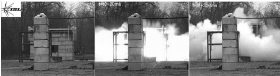
Effects of enhanced blast homemade explosives detonated inside building
