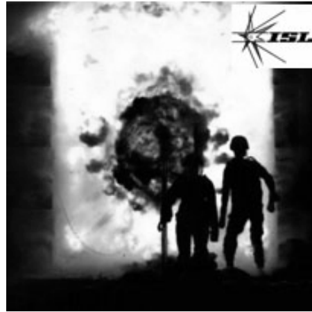
Effects on personnel of home-made charge detonated between 2 walls
