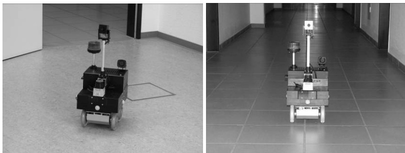
Fig. 1: SentryBots on patrol: Autonomous navigation within a self-generated map is one of the key aspects of the system.
