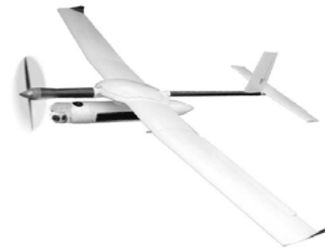
Figure 3. Rapidly deployable UAV, 5m wing span
