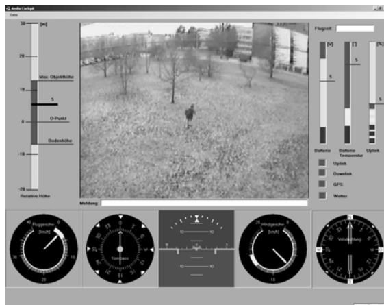
Fig 3: virtual cockpit for UAV control with display for on board video
