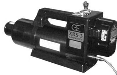
Figure 1: Portable X-ray source: flash generator by Golden Engineering
