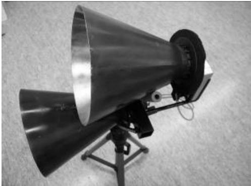
Fig. 2. Realization of optimized combined calorimetric sensor
