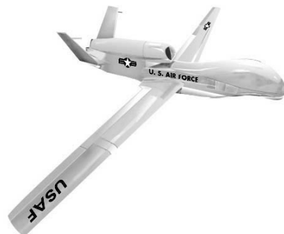
Figure 2. Long endurance UAV, 35m wing span
