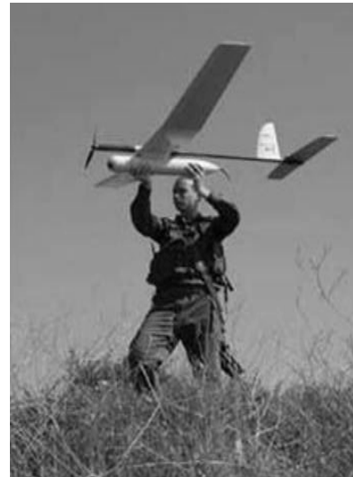
Figure 4. Shoulder launched UAV, 2,4m wing span
