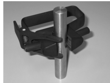
Figure 5: CIBA installed on a metallic bar
