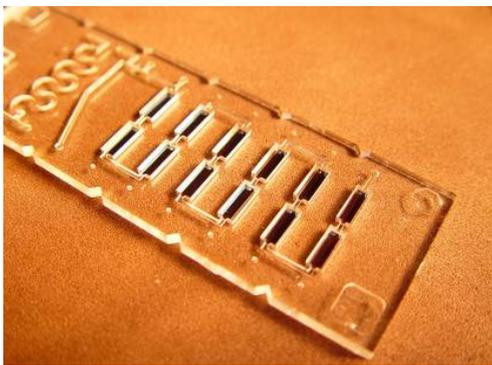
Figure 6.8a: Microfluidic chip with silicon die inserts for biological screening experiments.
