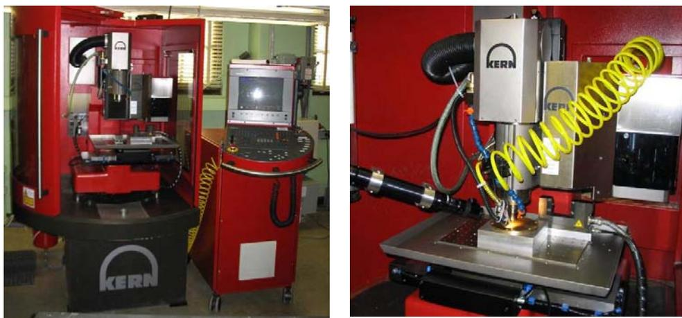
Figure 5.3: Kern<sup>®</sup> Micromilling Machine used to mill mold inserts in brass. The machine is operated and maintained by Jason Guy as part of the Center for Bio-Modular Multi-scale Systems (CBM<sup>2</sup>) under Dr. Steven Soper.
