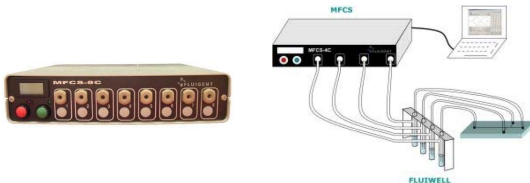
Figure 2.6a: Fluigent MFCS-8C flow controller (Left) uses air pressure to drive liquids and is capable of flow rates ranging from less than a nanoliter per minute up to hundreds of microliters per minute. Schematic (Right) shows the setup using such a system (Source: Fluigent’s website).
