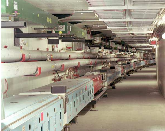
Figure 2.4: The Main Injector (light blue magnets at the bottom) and the Recycler (green magnets on top).
