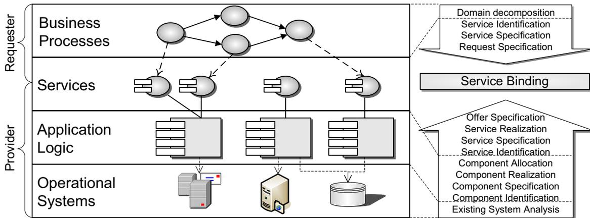
Figure 3.3: SOA layers and Web service engineering process
