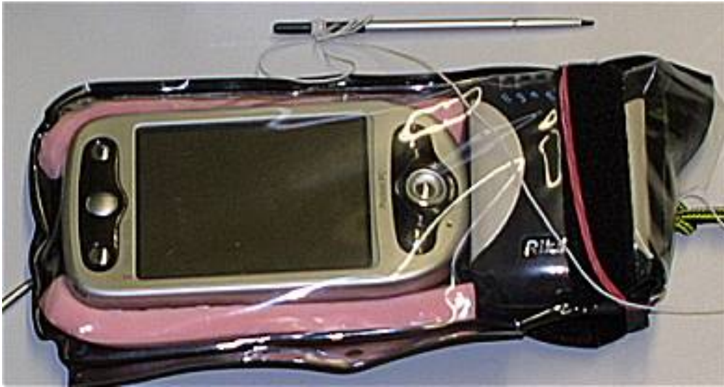
Figure 4.11: Hardware technologies employed for the MobiNaG prototype include a Pocket PC based PDA (left: here T-Mobile MDA II and stylus) and a BT GPS receiver unit (right: here Rikaline TM GPS-6031-X7) enclosed in protective casing for field test.
