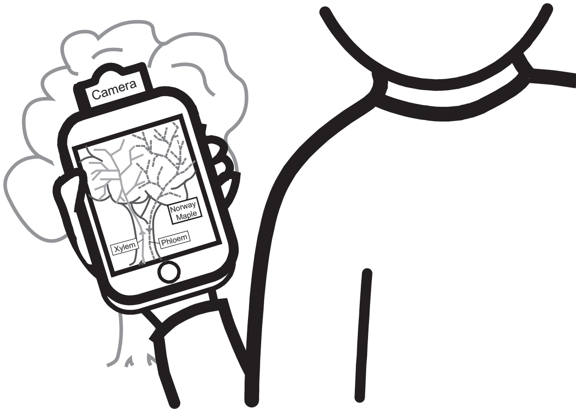
Figure 3.8: Based on a "video see-through" hand-held display the visitor's view of the environment (here a tree) can be superimposed with "augmented labels" and a "x-ray-vision" tool can augment the visual perception to reveal the vascular tissue inside the maple tree, which transports water from the roots to the canopy (i.e. xylem) and the tissue that transports soluble nutrients from the leaves down to other plant organs (i.e. phloem).
