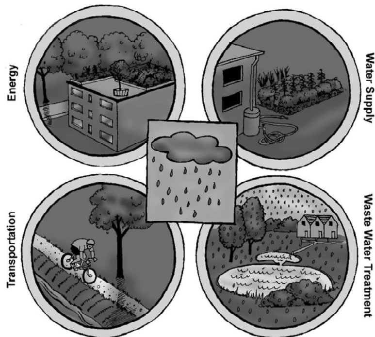
Figure 91 The One-system approach: storm water management features simultaneously serve to reduce energy demand, enhance transportation options, reduce demands for treated water, create local amenities and facilitate waste water treatment.
