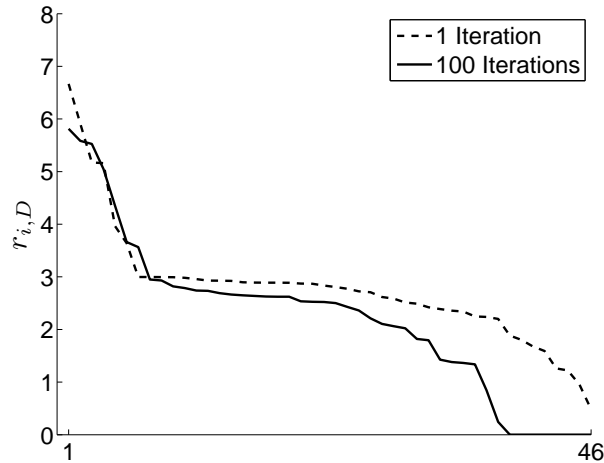
Figure 6.12: Behaviour of the redundancy numbers of the local-tie-solutions during iteration of variance components for the combination of solutions of different techniques, estimating variance components for both space geodetic solutions and local ties by the degree of freedom method. The values are sorted descendingly.
