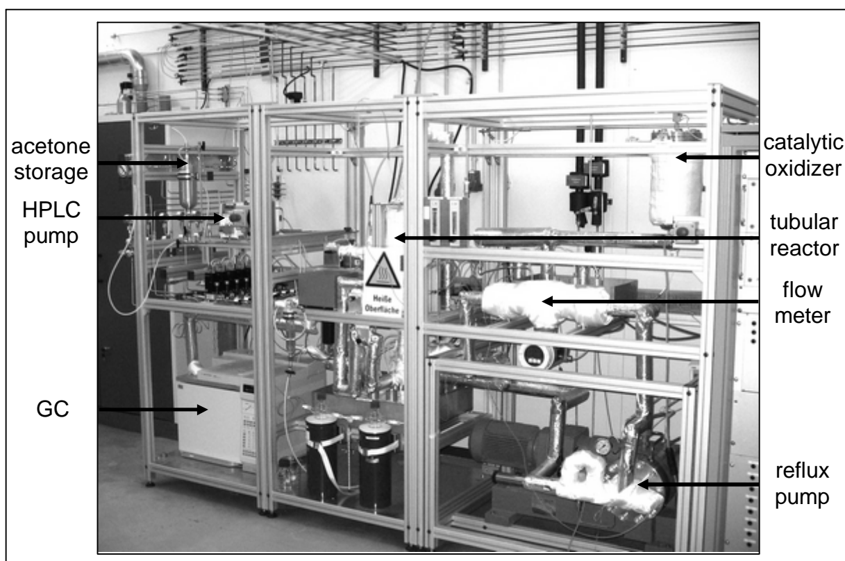
Figure 3.4: Image of the tubular reactor unit.
