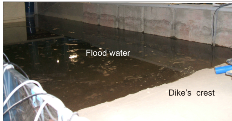
Figure 7.4: Flooding experiment at flood level 1.25 m. At this flood level the dike's crest was almost covered with flood water.
