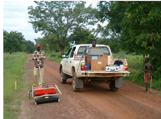
(b) Operation of GPR in CO mode
