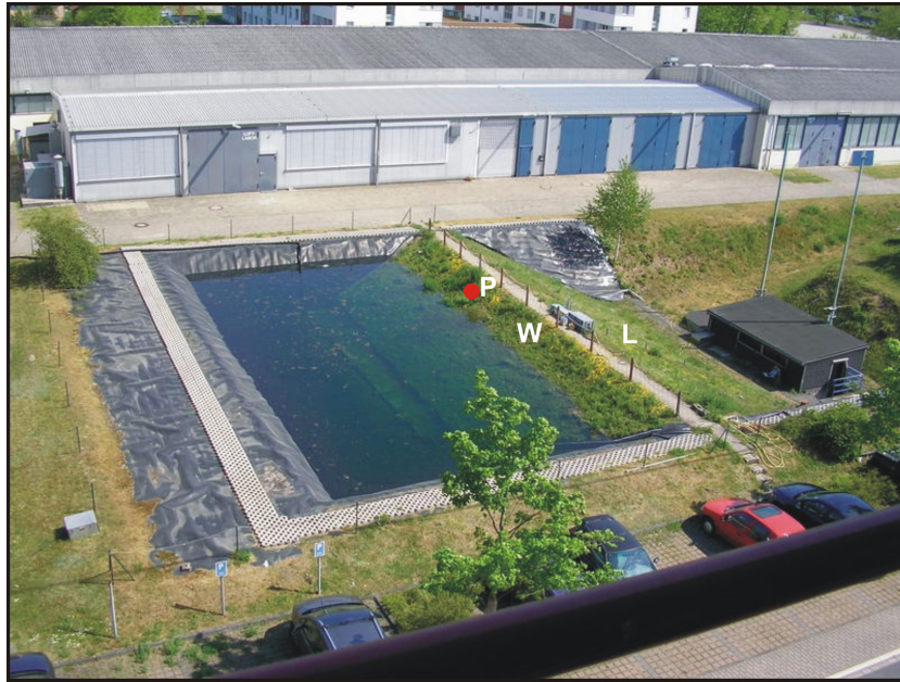
Figure 7.24: Dike model B of the Federal Waterways and Research Institute, Karlsruhe, Germany. Picture shows the data acquisition point of GWS (P), the waterside (W) and the landside (L) of the dike model.
