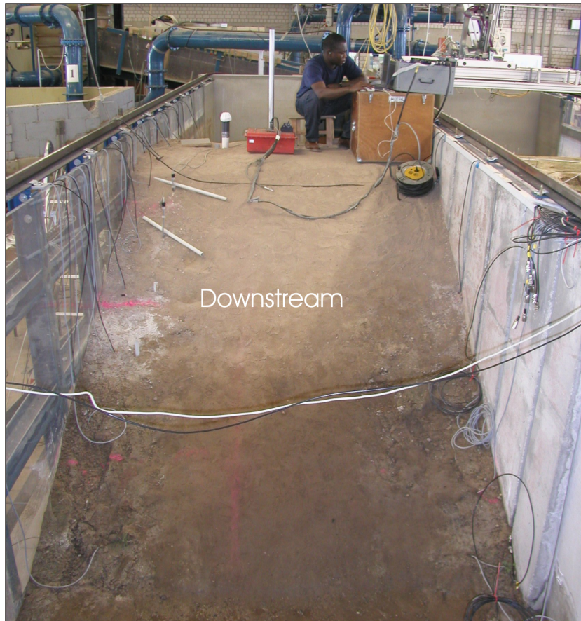
Figure 7.1: Dike model A at the Theodor-Rehbock-Laboratory, Institute for Water and River Basin Management, University of Karlsruhe, Karlsruhe, Germany. Picture shows the operation of the GPR in the GWS mode from the crest of the dike.
