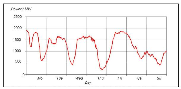
Figure 10: Wind energy production in the northem part of the E.ON-grid during the period Jan. 31<sup>th</sup> until Feb. 06<sup>th</sup>, 2000 [Luther et al. 2001].
