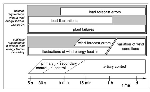
Figure 12: Reserve requirements in power systems with large wind energy feed-in (adapted from [Dany 2000])
