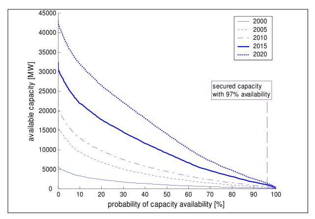
Figure 38: Secured wind power capacity (good wind year) in Germany as a function of capacity availability, derived from AEOLIUS wind power time series
