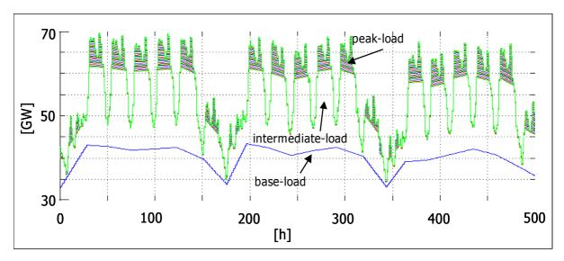
Figure 24: Load coverage by base, intermediate, and peak load capacities
