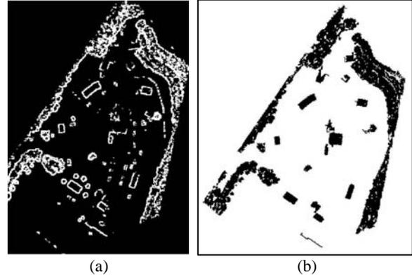
Figure 4: a) Detection of the off-terrain class borders ( $\Delta h=3$  m). b) Detected off-terrain objects ( $\Delta h=3$  m and  $S=75$  m<sup>2</sup>).
