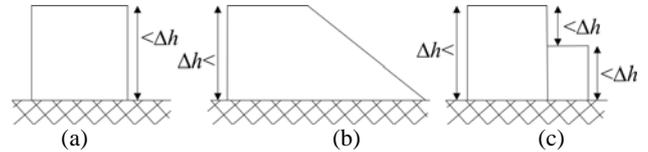
Figure 5: Three cases for the non-detection of building boundaries: a) Building with a height smaller than  $\Delta h$ . b) Building with an inclined facade. c) Building with an obstacle in the vicinity.
