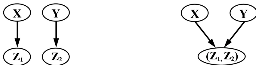
Figure 4.8.: A coarse-grained structure \mathcal{G}_1 (right plot) is obtained by merging distinct nodes Z_1 and Z_2 of a fine-grained structure \mathcal{G}_0 (left plot) to a two-dimensional variable Z := (Z_1, Z_2) . Both describe consistent manipulation potentials (see Eq. (1.3) for manipulation criterion), however, do not share the same feature with respect to the independence relations between X and Y conditional on (Z_1, Z_2) .
