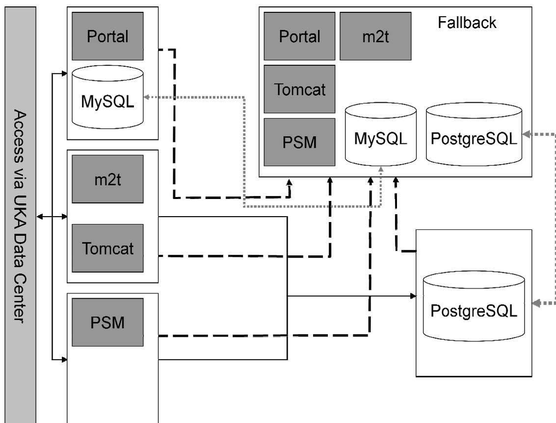
**Figure 11: Hardware and software architecture of STOCCER**
