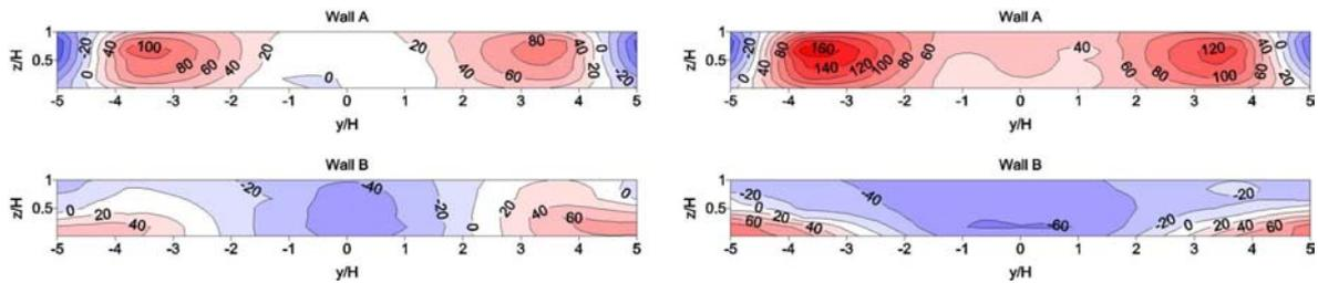
Figure 3. Relative changes in concentration for tree planting with spacing 30 m (left) and spacing 15 m (right) when compared to the reference case (Figure 2).
