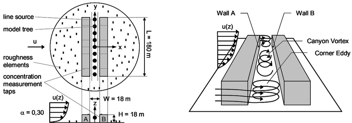
Figure 1. Model setup and flow field inside empty street canyon of aspect ratio  $H/W = 1$ .
