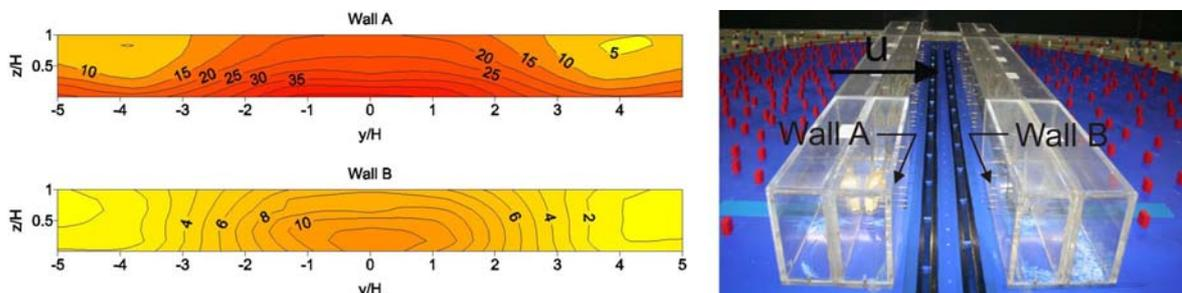
Figure 2. Normalized wall concentrations for empty street canyon without trees (reference case).
