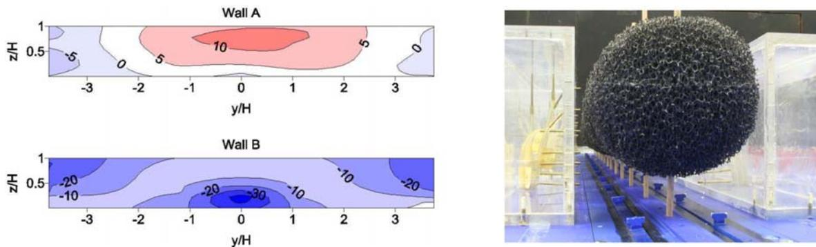
Figure 4. Relative changes in concentration for tree planting with spacing 15 m and permeable crowns when compared to tree planting with impermeable crowns.
