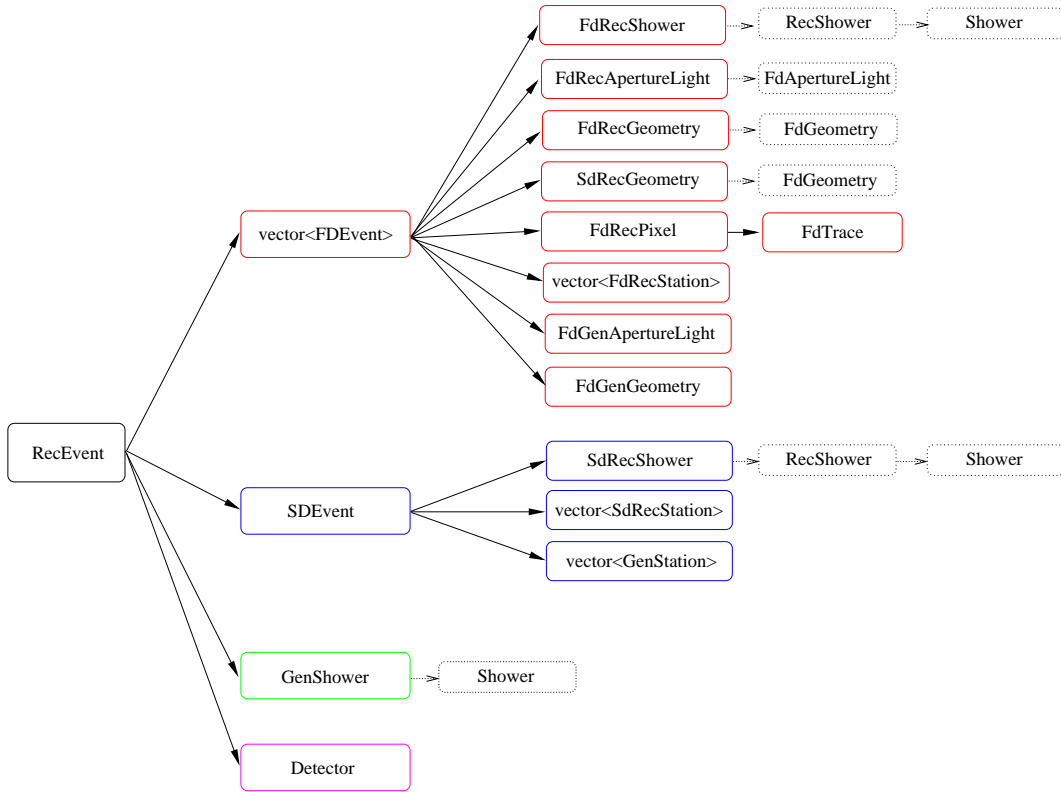
Figure 3.15: Layout of the ADST data containers to store reconstructed as well as simulated event information.
