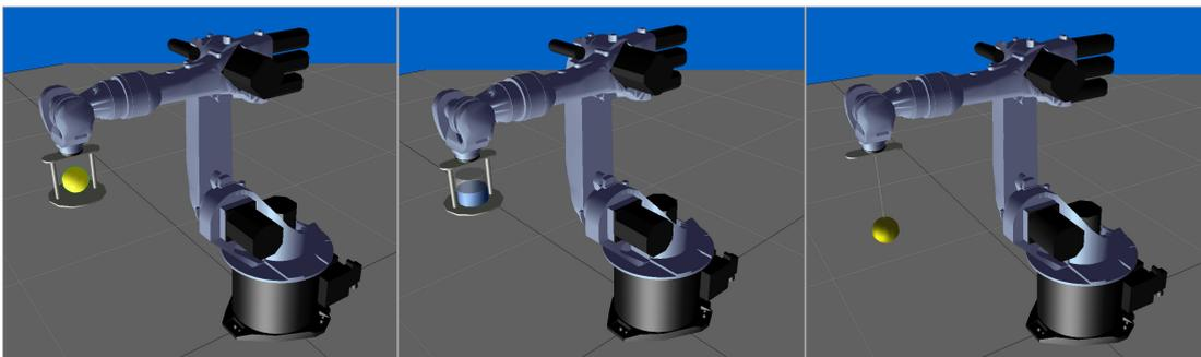
Fig. 1-3: Three problem-scenarios in evaluation. Minimizing of shear forces (a), liquid sloshing (b) and sway oscillations (c).
