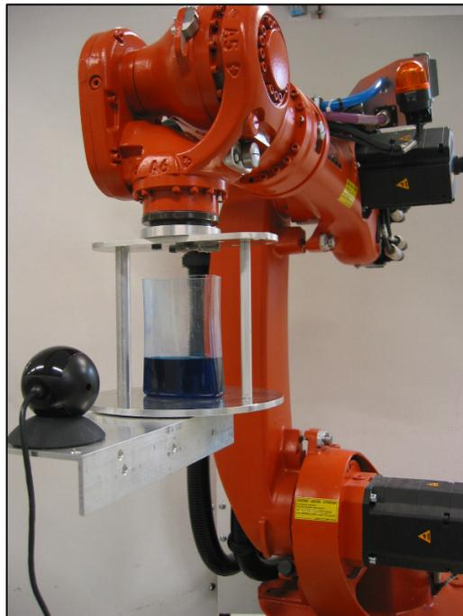
**Fig. 5-8: Industrial manipulator (6 DOF) with the carrying tool, the test-recipient with coloured water and the sensor camera.**
