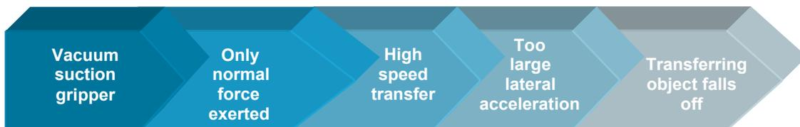
Fig. 4-2: Problem encountered commonly by using vacuum suction grippers.
