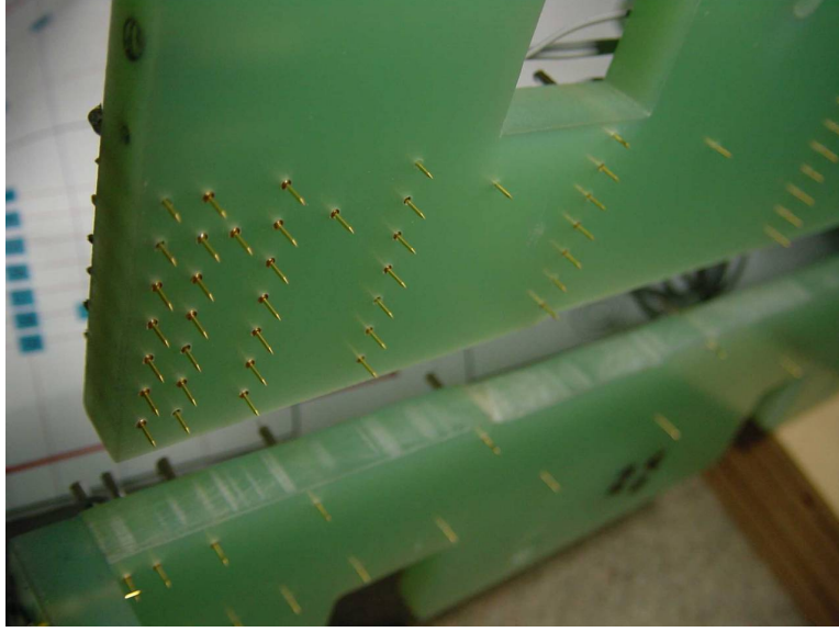
Figure 77: Photograph of an insulating plate showing sensing spring-loaded needles.
