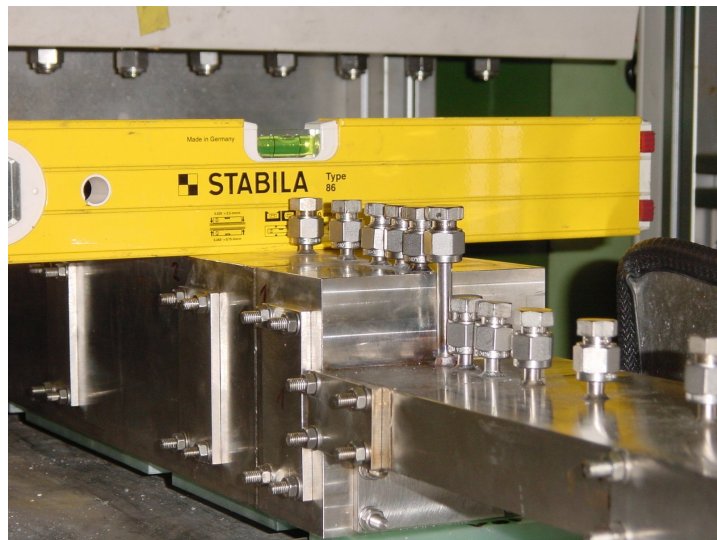
Figure 34: Test section during installation into the liquid-metal loop. All pressure taps are closed.
